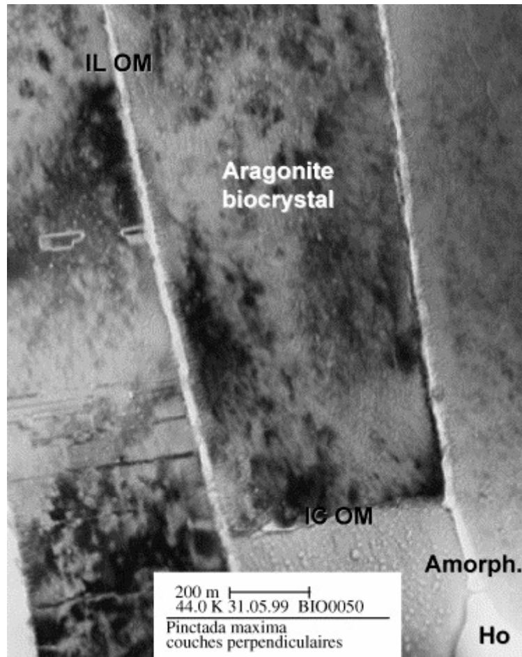
Fig. 5. Contrasted brightfield TEM image showing the aragonite biocrystals (Ho: hole, Amorph.: amorphized area, ICOM: intercrystalline organic matrix, ILOM: interlaminar organic matrix).
