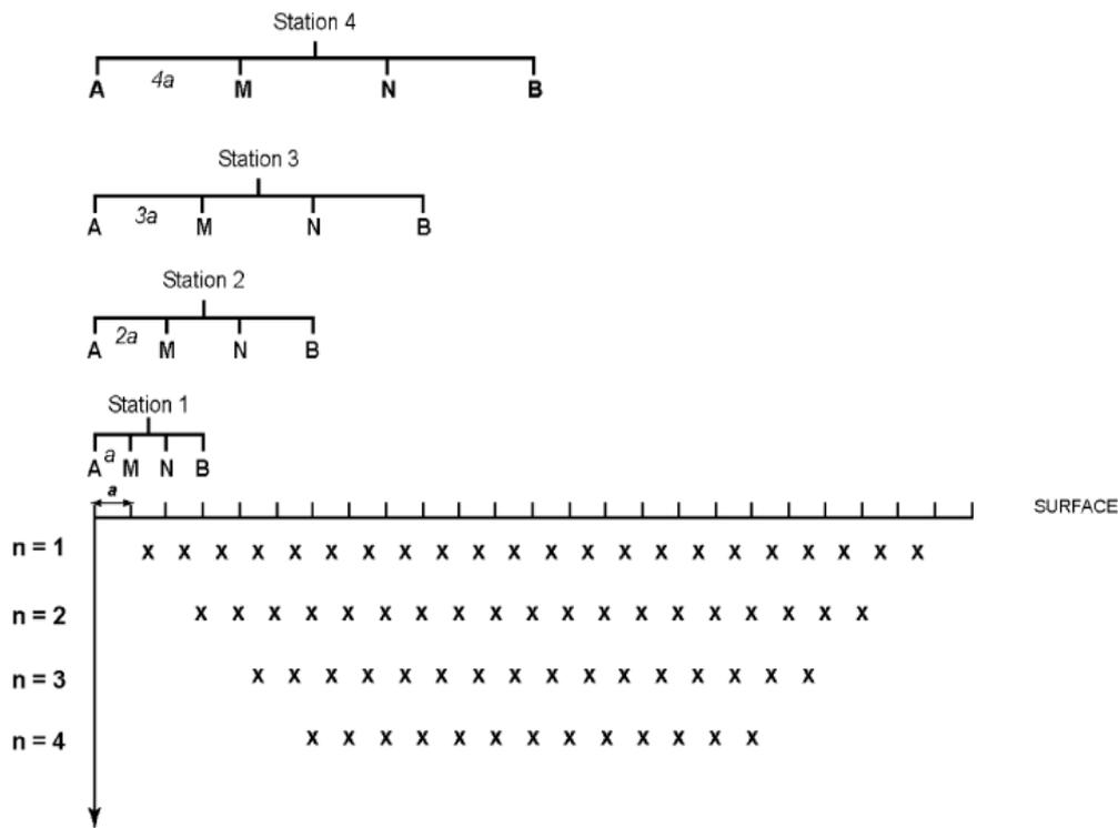
Fig. 4. Establishment of a 2D electrical resistivity pseudo-section.
