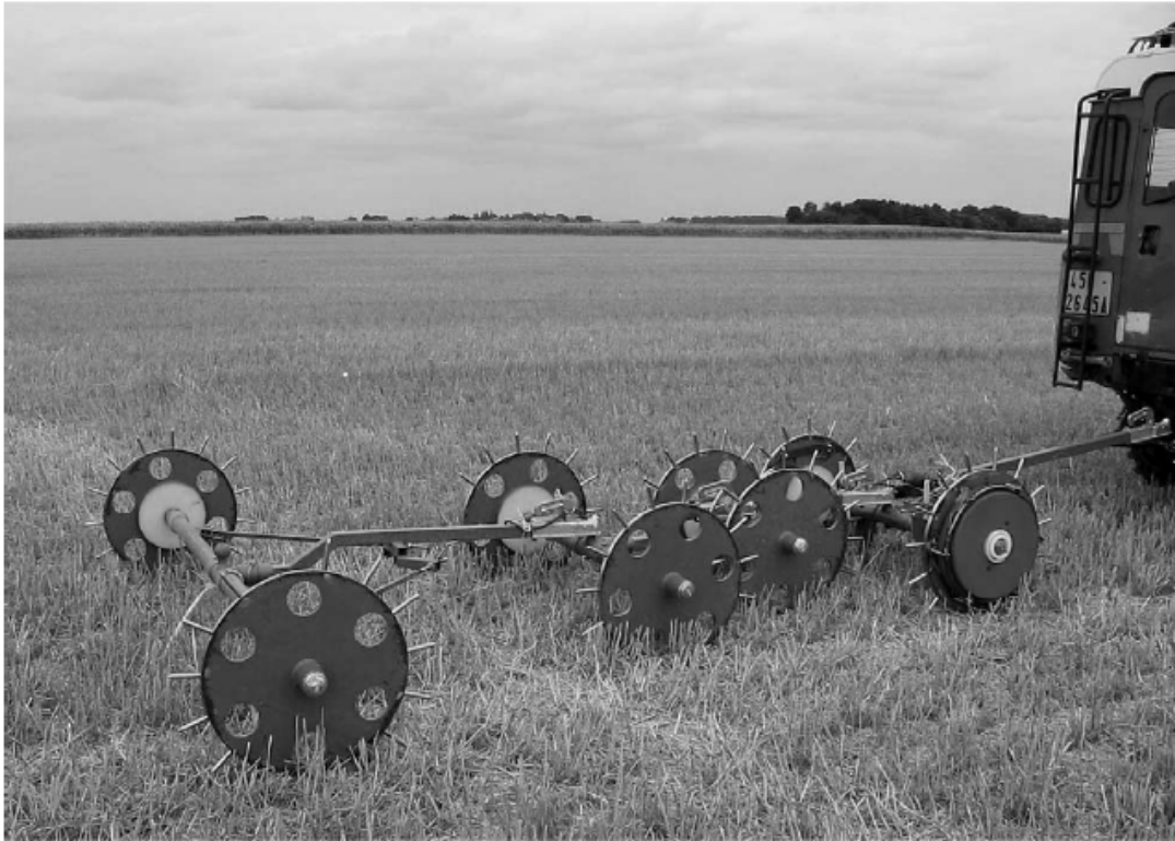
Fig. 5. Multidepth Continuous Electrical Profiling (MUCEP).
