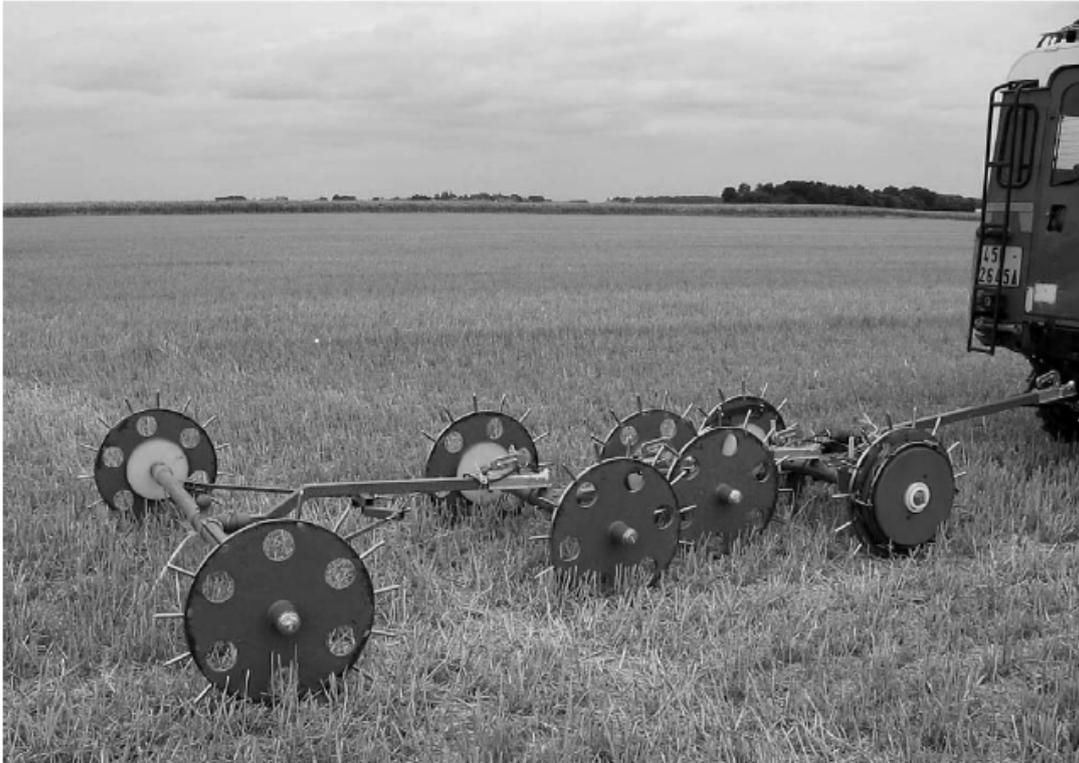
Fig. 5. Multidepth Continuous Electrical Profiling (MUCEP).
