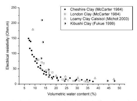
Fig. 2. Relationship between the volumetric water content and the electrical resistivity for different soil types (values issues from Fukue et al., 1999; Michot et al., 2003; McCarter, 1984).
