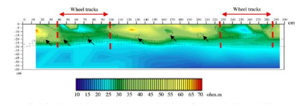
Fig. 8. Two-dimensional electrical resistivity image perpendicular in the traffic direction (after Besson et al., 2004).
