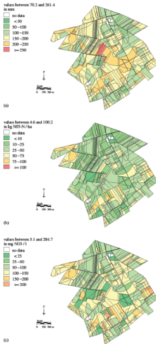
Figure 5. Simulation maps of mean annual values over the period 1991–1998 of: (a) cumulative water drainage, (b) cumulative N leaching, and (c) nitrate concentration in drainage water. Black lines are the borders of the SU.
