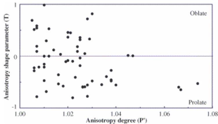
Fig. 5. Plot of anisotropy degree ( $P'$ ) vs. anisotropy shape ( $T$ ) of magnetic susceptibility.  $P' = \exp\{2[(\ln K_1 - \ln K_m)^2 + (\ln K_2 - \ln K_m)^2 + (\ln K_3 - \ln K_m)^2]^{1/2}\}$ , and  $T = [2 \ln(K_2/K_3) / \ln(K_1/K_3)] - 1$ , where  $K_1$ ,  $K_2$  and  $K_3$  are principal axes of the magnetic fabrics and  $K_m$  is their average.
