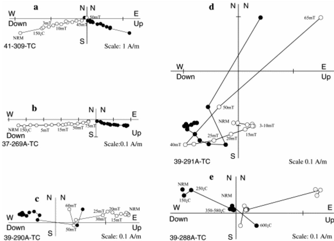
Fig. 3. Orthogonal projection in tilt-corrected coordinates of progressive demagnetization for representative samples (Zijderveld, 1967). Black (whites) dots present horizontal (vertical) plans.
