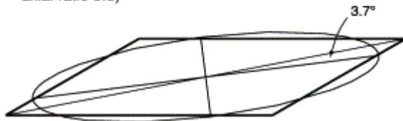
e) Type 2 monoclinic particle (NIH best fit ellipse axial ratio 4.4, weakly oblique to diagonal)
