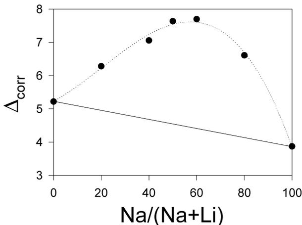
FIGURE 7. Variation in line width ( $\Delta_{\text{corr}}$ ) measured for the 3600–3625  $\text{cm}^{-1}$  stretching region for synthetic amphiboles along the ferri-clinoferroholmquistite-riebeckite join.
