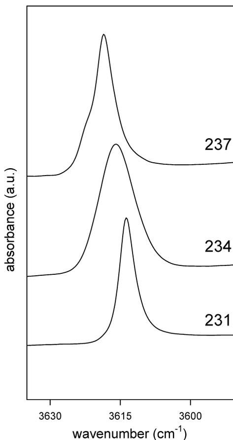
FIGURE 6. Enlargement in the 3630–3600 cm<sup>-1</sup> region for selected amphiboles along the ferri-clinoferroholmquistite-riebeckite join.
