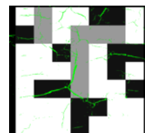
99 Figure 3 : Crack detection and orientation for the first pseudo-depth evaluated by 100 the AI The white represented the no-cracking area, the grey and light grey
