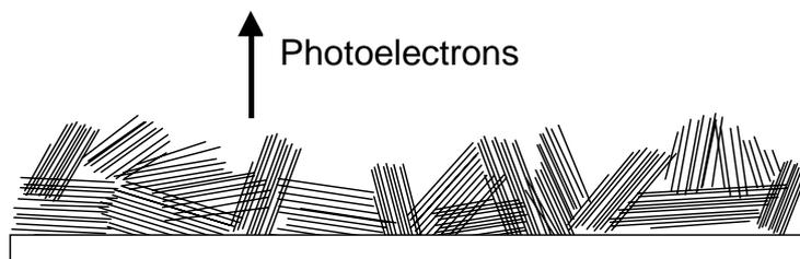
Figure 9. Schematic representation of the microstructural units of Prrenjas bentonite, with numerous edge-face associations of particles, showing the significance of edge surfaces for XPS analysis.
