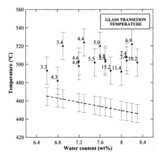
Fig. 4. Glass transition temperatures ( $T_g$ ) as a function of the final water content. The plain triangles are the observed  $T_g$  ( $\pm 15^{\circ}$ C) labelled with the final pressures in kbar. The dots are the  $T_g$  ( $\pm 10^{\circ}$ C) calculated after [33] at atmospheric pressure for a cooling rate of 32°C/s. The dashed line is the best linear fit of the calculated  $T_g$ .
