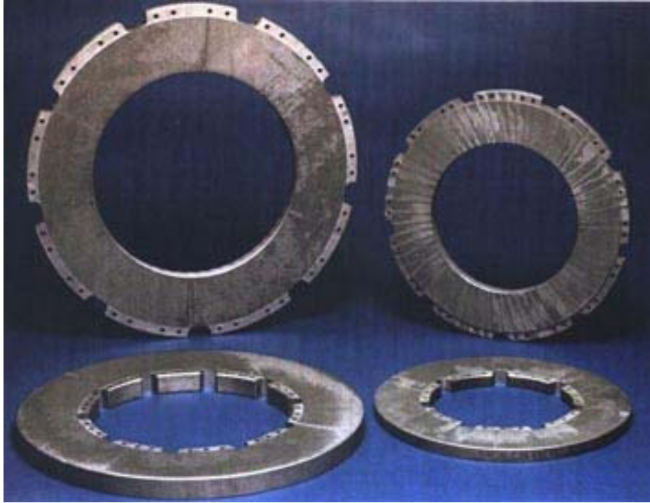
Figure 1 Aircraft brake disks (rotor and stator) made of carbon fiber-reinforced pyrocarbon.
