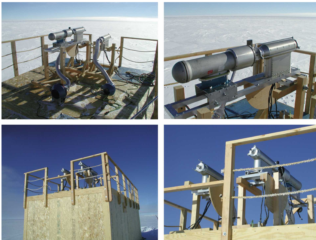
FIG. 1. Photographs of the SPEC CPIs and LaMP PN on top of a small building at the South Pole. The PN is seen connected to the exhaust region of the CPI in the panel at the upper left. Both instruments are aspirated using an exhaust fan. The sampling elevation is approximately 3 m.
