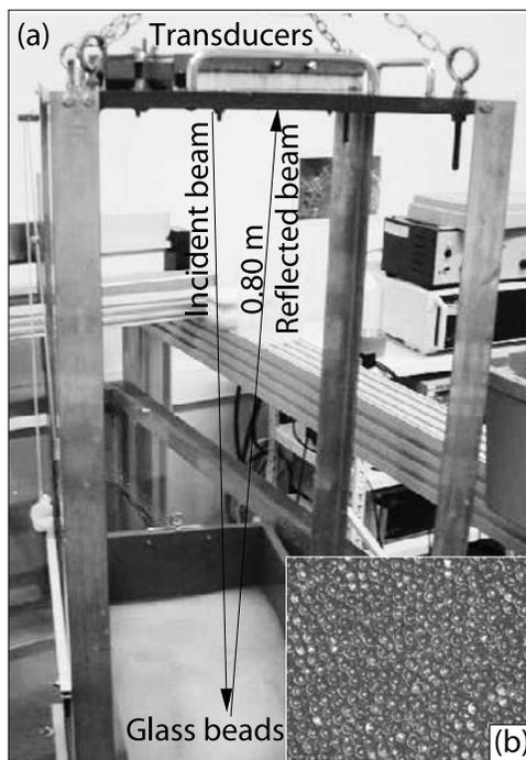
**Figure 2.** (a) Experimental setup holding two piezoelectric transducers above a rolling box filled with glass beads. The box can be horizontally translated while stacking the reflected signals in order to record the mean field. (b) Monodisperse glass beads randomly distributed in water. The concentration  $\phi \simeq 0.63$  roughly corresponds to  $10^9$  beads/m<sup>3</sup> for  $d = 1$  mm.
