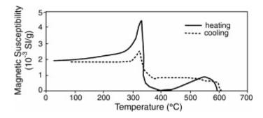
Fig. 10. Thermomagnetic profiles of the pyrrhotite ore.
