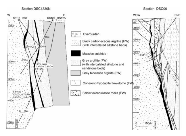
Fig. 3. Vertical east—west cross sections looking north through the Draa Sfar deposit showing the main ore zones and mine stratigraphy. To improve clarity, the mafic dykes and sills are not shown.
