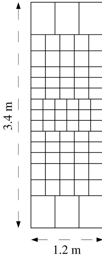
**Figure 7.** Discretization of the 2-D medium between the two boreholes: the size of the cells is set in order to homogenize the resolution, based on the density and orientation of the rays and on the resolving kernels shown in Fig. 6.
