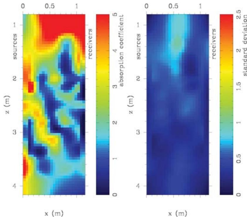
**Figure 11.** Interpolated model of attenuation coefficient between the two boreholes. Left-hand side: average values obtained from 50 likely models (high attenuation values are displayed in red while low attenuation values are displayed in blue). Right-hand side: standard deviation to the mean values. Note that the range of the colour scale used to represent the average model is twice larger than the one used to represent the standard deviation.
