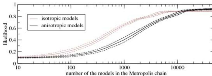
**Figure 9.** Likelihood curves of the models forming the Metropolis chain. The average curve of 50 isotropic inversions is plotted in grey solid line with its variability  $\pm \sigma$  (the standard deviation) plotted in grey dashed lines, the average curve of 50 anisotropic inversions and its variability are plotted in black solid and dashed lines.
