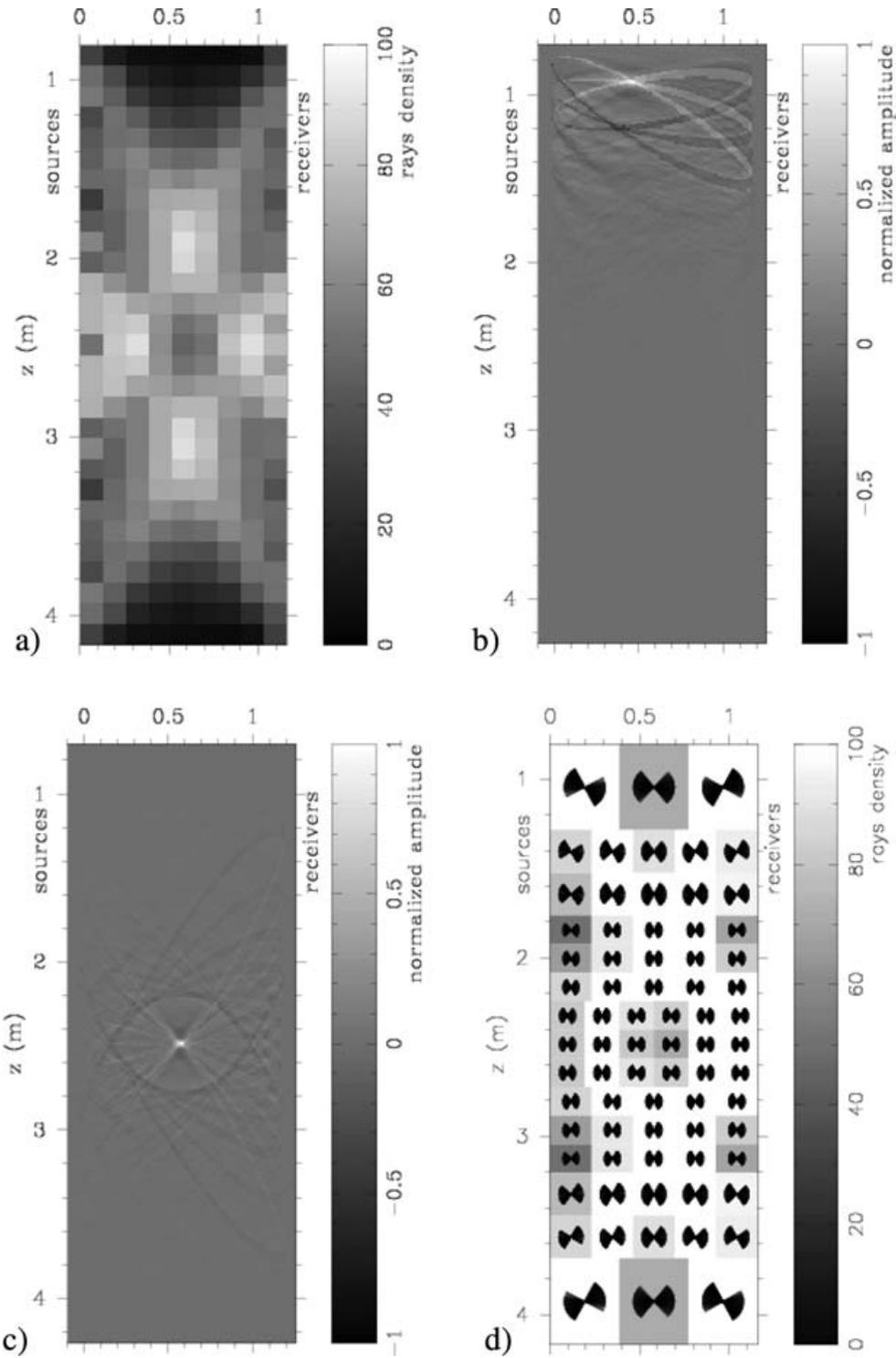
**Figure 6.** Lighting of the medium assuming straight ray paths: (a) ray-coverage density calculated on a regular grid of 9 per 29 rectangular cells; (b) and (c) two of the 261 (9 × 29) resolving kernels computed taking into account the Fresnel zone and (d) density and orientation of the rays in varying meshes whose size is optimized.
