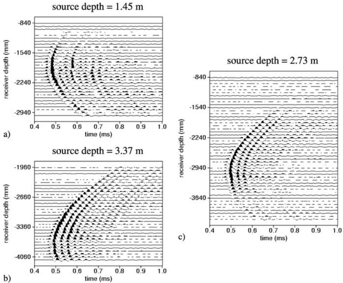
**Figure 3.** Raw data of the transmission tomography experiment gathered in common-shot for three source locations: (a)  $z_S = 1.45$  m recorded by the 32 higher receivers; (b)  $z_S = 3.37$  m recorded by the 32 lower receivers and (c)  $z_S = 2.73$  m recorded by the 48 receivers.
