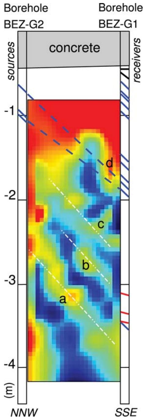
**Figure 13.** Sketch of the different structural features observed and expected in the tomographic domain. The oblique lines drawn in the two boreholes correspond to fractures observed in the extracted cores. The dashed lines drawn between the boreholes are hypothetical tectonic fractures. The tomographic image of the maximum attenuation of the anisotropic model is shown for comparison (same colour scale as in Fig. 12a).
