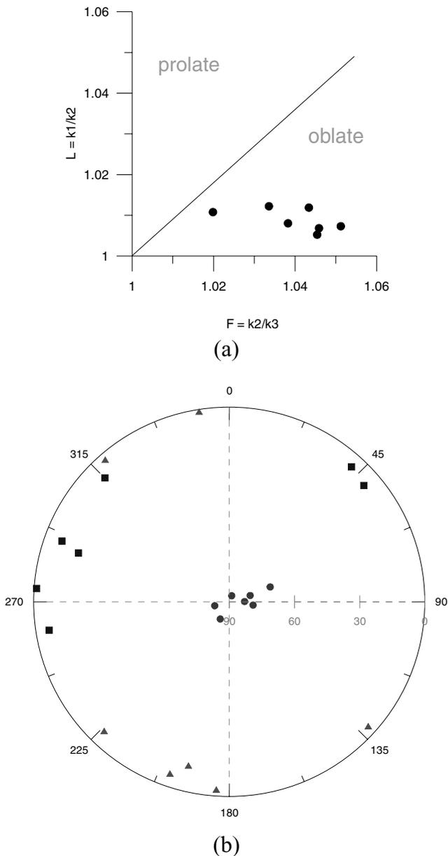
**Figure 7.** (a) Flinn-type plot of the degree of lineation ( $L$ ) and foliation ( $F$ ), (b) equal-area projection of the principal axes of magnetic susceptibility ellipsoid (Vagnari kiln). Symbols: square = maximum; triangle = intermediate; dot = minimum axis of susceptibility.
