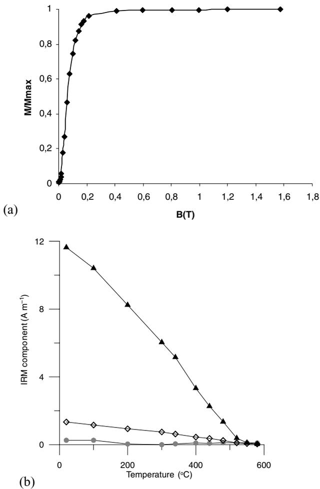
**Figure 4.** (a) Isothermal remanent acquisition (IRM) curve (b) thermal demagnetization of IRM components (specimens from the structures Nos. 14 and 3—Table 1). Symbols: black triangle = low-; open diamond = intermediate-; grey dot = high-coercivity component.
