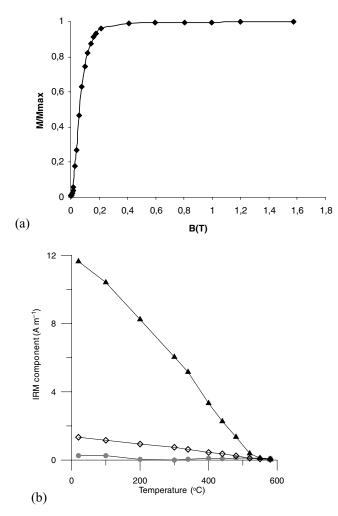
**Figure 4.** (a) Isothermal remanent acquisition (IRM) curve (b) thermal demagnetization of IRM components (specimens from the structures Nos. 14 and 3—Table 1). Symbols: black triangle = low-; open diamond = intermediate-; grey dot = high-coercivity component.
