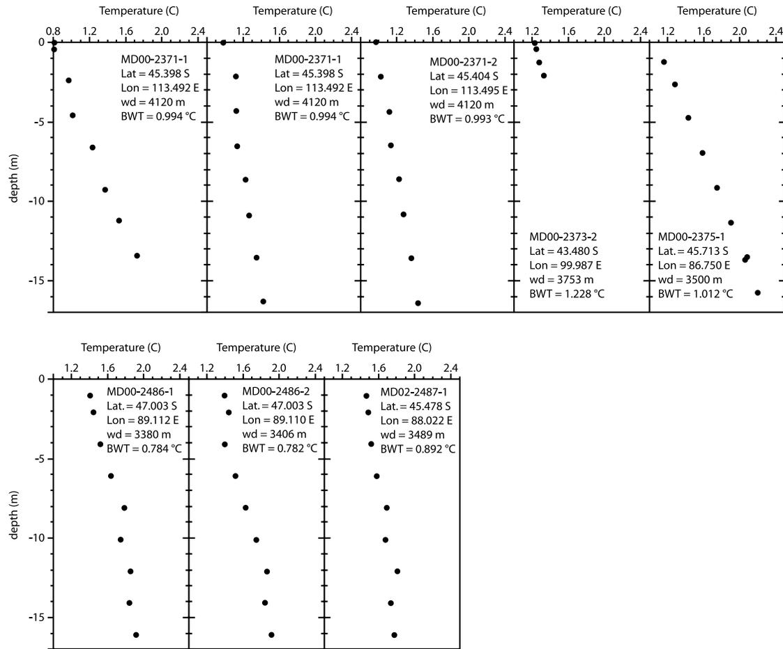
**Figure 8.** Temperature profiles obtained with R/V *Marion Dufresne* on the southern flank of the SEIR (see Table 1). The sediment equilibrium temperature was obtained using the classical method [Langseth, 1965].
