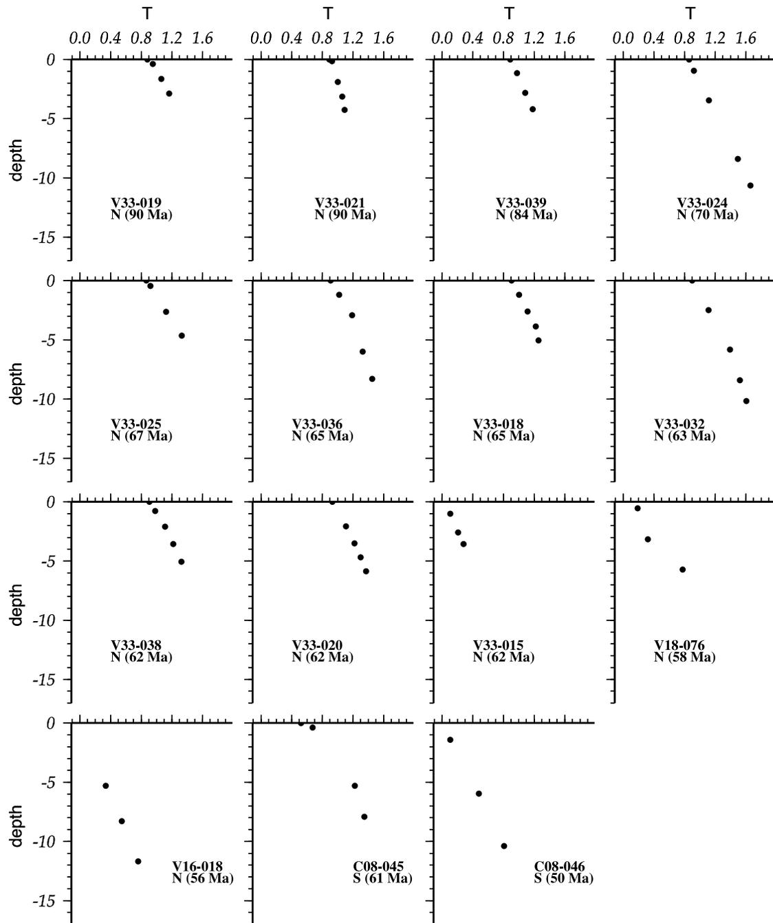
**Figure 5a.** Sediment temperature ( $^{\circ}\text{C}$ ) profiles versus depth from the LDEO database for data points from the crust older than 43 Ma. Depths are in meters below seafloor (assuming full probe penetration). N and S indicate north and south flanks, respectively.
