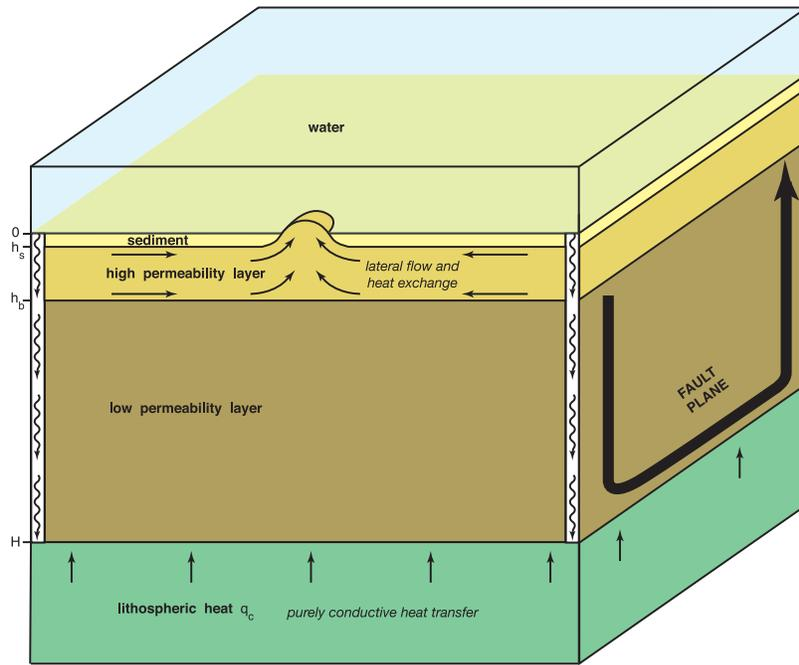
**Figure 11.** Cartoon for the hydrological model. Seawater circulation within the upper crustal layer is horizontal and controlled by basement topography. Within the lower crustal layer, seawater may occur along faults planes (ridge-parallel and ridge-perpendicular), down to the base of the crust.
