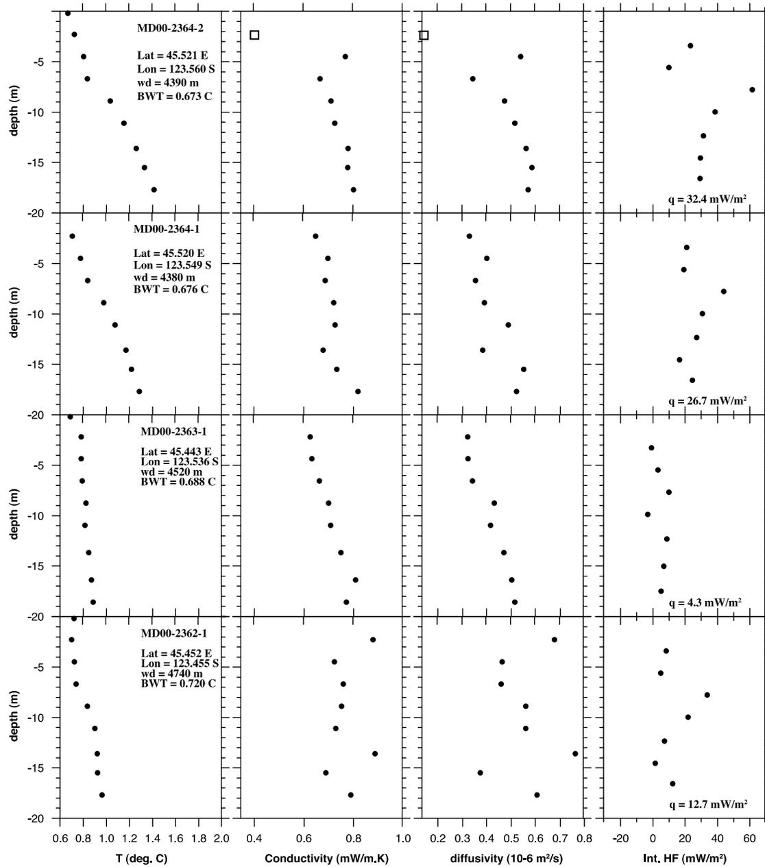
**Figure 7.** Thermal measurements obtained with R/V *Marion Dufresne* on the northern flank of the SEIR (see Table 1). The equilibrium temperature, the thermal conductivity, and the thermal diffusivity of the sediments were obtained by inverse modeling the first minute of the cooling curve (temperature versus time) after the penetration of the core.
