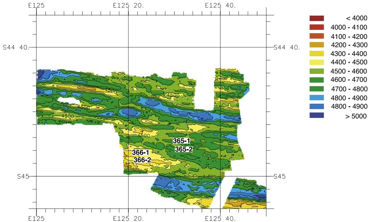
**Figure A3.** Same as Figure A1 except for bathymetry in the vicinity of sites 365-1, 365-2, 366-1, and 366-2. The measured values of heat flow (4 and 7  $\text{mW m}^{-2}$ ) over the topographic high (MD00-366) are smaller than those (46 and 36  $\text{mW m}^{-2}$ ) found at site MD00-2365 over in the topographic lows, opposite to the trend in Figures A2 and A4.
