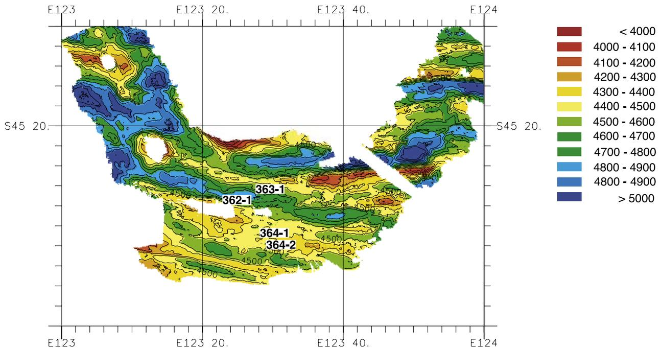
**Figure A2.** Same as Figure A1 except for bathymetry in the vicinity of sites 362-1, 363-1, 364-1, and 364-2. The measured values of heat flow (13 and 4  $\text{mW m}^{-2}$ ) over the topographic lows (MD00-362 and MD00-363) are smaller than those (32 and 44  $\text{mW m}^{-2}$ ) found at site MD00-2364 over topographic highs.
