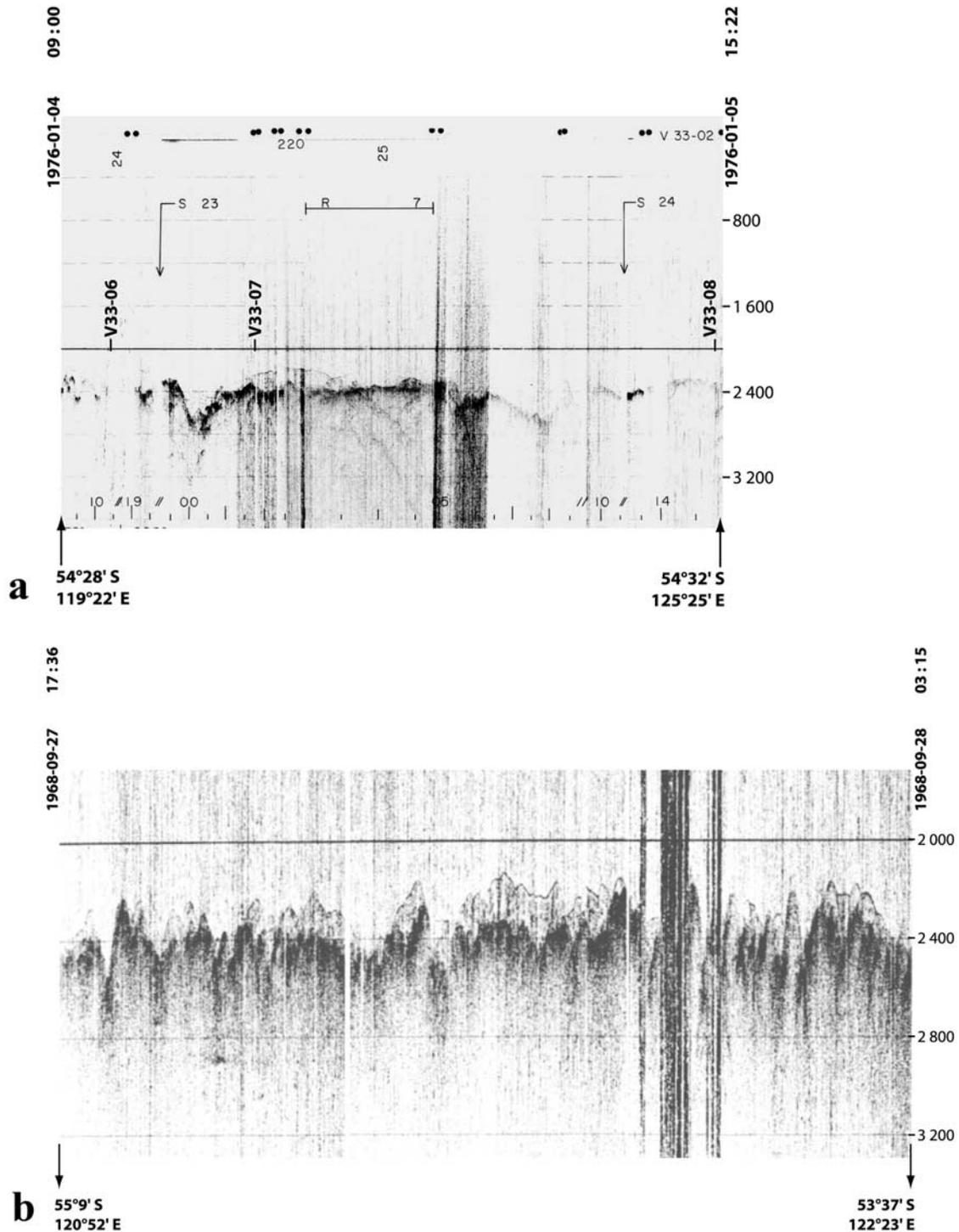
**Figure 3.** Selected seismic sections from the southern flank (see profile locations in Figure 2). (a) Line V33-02, with location of heat flow sites V33-06, V33-07, and V33-08. Note that the seismic acquisition was interrupted between sites V33-06 and V33-07, which are spaced  $\sim 200$  km apart. (b) Section ELT035-55. The depth scale on the right is in fathoms (1 fathom = 1.83 m). Original seismic images are available on line at <http://www.marine-geo.org/seislink>.
