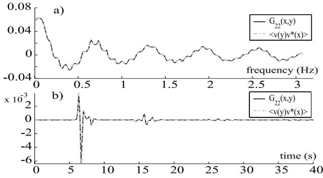
**Figure 2.** (a) Solid black line depicts the imaginary part of the Green function. The dashed gray line is the average cross-correlation between the displacements recorded at points  $\mathbf{x}$  and  $\mathbf{y}$ . (b) The solid black line is the synthetic seismogram generated by the analytical Green function. The dashed gray line represents the synthetic seismogram generated by the cross-correlation and its Hilbert transform.
