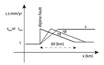
**Figure 1.** Tectonic models adopted here. Here r is the vertical rock uplift velocity function; s is the horizontal advection velocity function; rA depicts the case where the maximum rock uplift is near the fault; and rB is where the maximum rock uplift is away from the fault.
