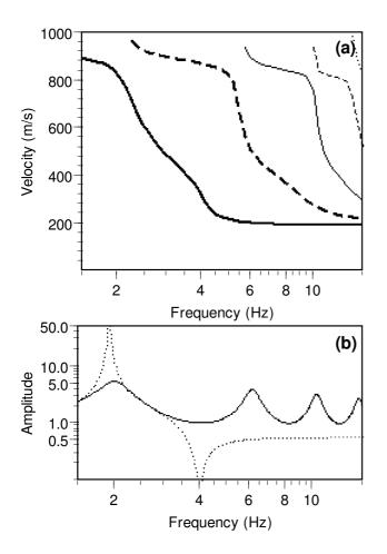
Figure 3: Synthetic model. (a) Dispersion curves for Rayleigh modes: fundamental mode (thick plain line), first (thick dashed line), second (thin plain line), third (thin dashed line), and fourth higher modes (thin dotted line). Other modes do not exist in the plotted range. (b) Fundamental Rayleigh ellipticity curve (dotted line) and theoretical  $S_H$  transfer function for the synthetic model (plain line).
