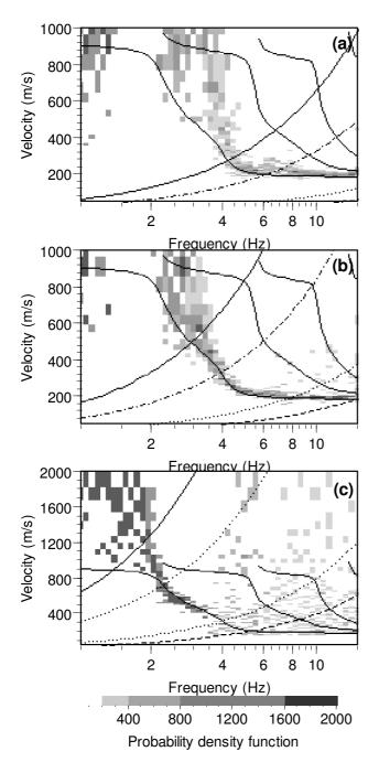
Figure 6: Frequency-wavenumber method applied to arrays A (a), B (b) and D (c) with time windows of 50 cycles as in Figure 5(b). The histograms and the curves are of the same type as in Figure 5.
