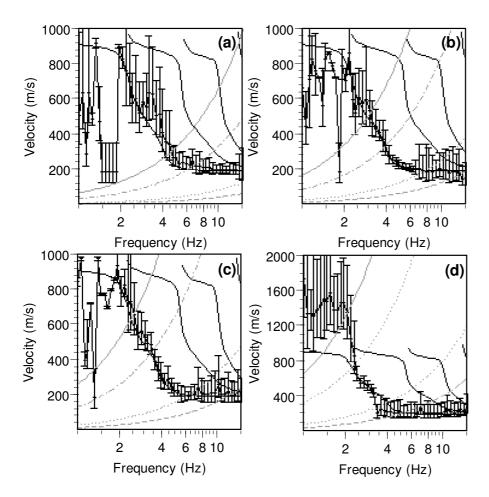
Figure 8: Dispersion curves derived from the high resolution frequency-wavenumber method applied to arrays A (a), B (b), C (c) and D (d). The black lines with dots and error bars, obtained from computations, are compared to the theoretical dispersion curves (thin plain lines). The gray exponential curves are similar to the ones in Figure 5.
