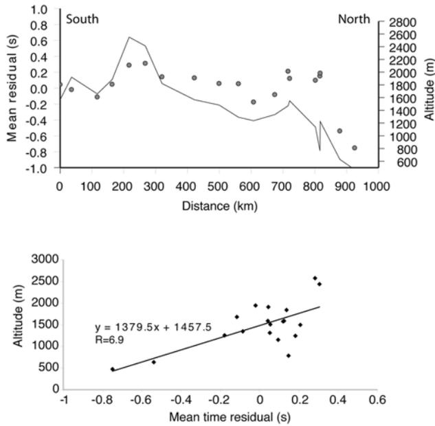
**Figure 2.** (top) Mean traveltime residuals (left scale, grey dots) and station elevation (right scale, solid line) across the MOBAL profile. (bottom) Correlation between topography and traveltime residuals. The slope should be indicative of the mantle P-wave velocity if the B factor relating velocity with density is constant through the model.
