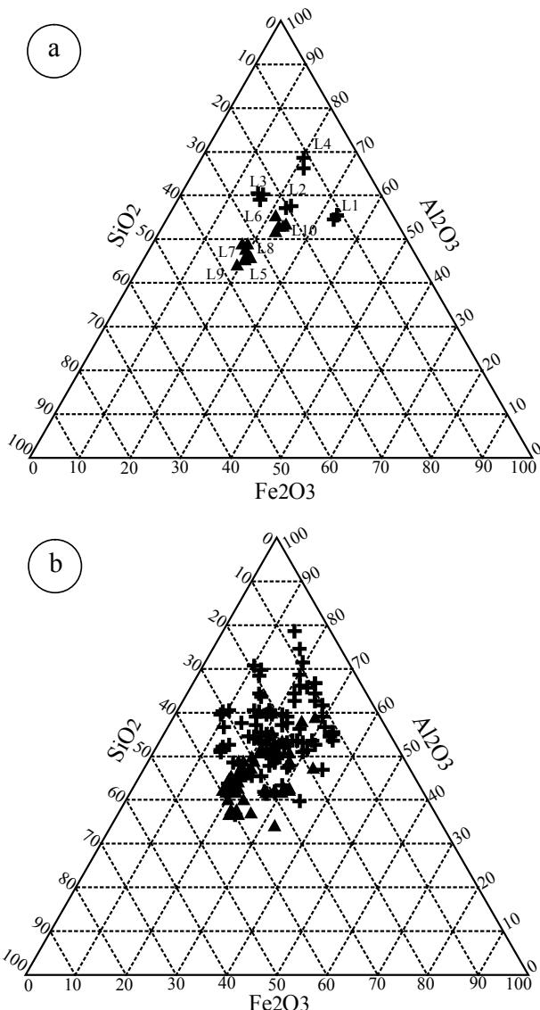
Fig. 1.  $\text{SiO}_2$ ,  $\text{Al}_2\text{O}_3$  and  $\text{Fe}_2\text{O}_3$  relative contents in the Bw horizons of the Latosols of the regional toposequence studied (a) and those of Bw horizons from the literature (b): Latosols located on the South American Surface (+) and Velhas Surface ( $\blacktriangle$ ).
