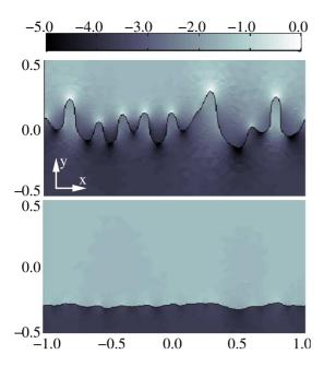
FIG. 2: (Color online) Map of the logarithm of the elastic energy in the solids during the roughening process, with  $E_1 = 10$  GPa,  $E_2 = 60$  GPa,  $\nu_1 = \nu_2 = 0.3$ , and  $\sigma_0 = 0.05$  MPa. Lower panel: initial h(x) at t = 0. Upper panel: interface at a later stage of roughening.
