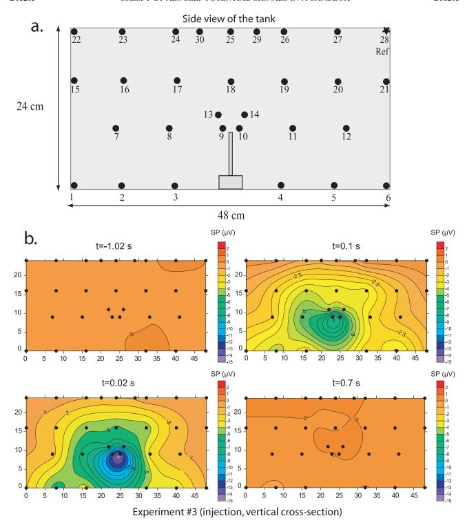
**Figure 7.** Injection experiment (Experiment #3). (a) Side view of the tank with the position of the electrodes (#28 is the reference) and the position of the capillary. (b) Snapshots of the electrical potential distribution of the self-potential at four different time-lapses. The shock created by the hammer stroke is smaller than in Experiment #1.
