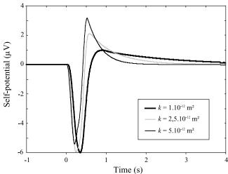
**Figure 16.** Simulated self-potential response at electrode #32 for different values of the permeability *k* (Experiment #1).
