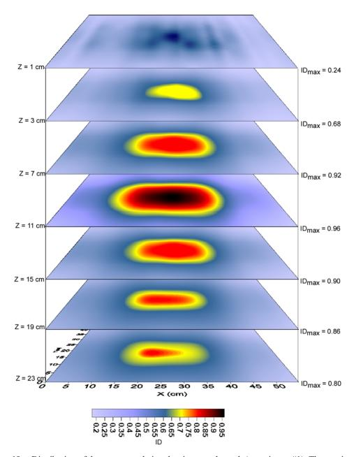
**Figure 19.** Distribution of the cross-correlation density over the tank (experiment #1). The maximum of the cross-correlation distribution is located at a depth of 14 cm below the top surface of the tank. The numbers on the right side of the tomogram represent the maxima of the cross-correlation function for each horizontal plane.
