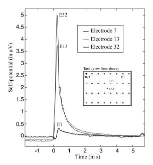
**Figure 6.** Electrograms for some selected electrodes (Electrodes E7, E13, and E32) located in the vicinity of the top surface of the tank during the pumping experiment (Experiment #2). There is no change of the polarity during the course of the experiment.
