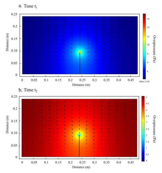
**Figure 13.** The arrows show the direction of the total displacement  $\mathbf{u}$  (in m) at time  $t_1$  (a) and at time  $t_2$  (b) respectively (see Figure 14). The colors code the fluid pressure above hydrostatic (in Pa). The change of polarity is due the reversal of the fluid flow due to the boundary condition expressed in term of fluid pressure at the end of the capillary. This polarity change is entirely due to the piston-like effect of the syringe.
