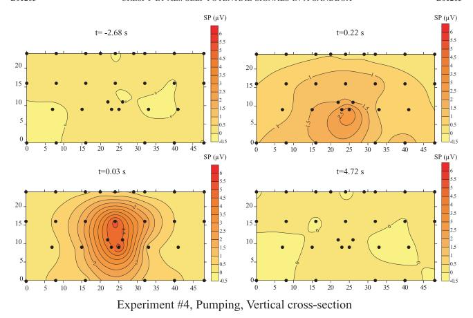
**Figure 9.** Pumping experiment (Experiment #4). Snapshots of the electrical potential distribution of the self-potential at four different time-lapses. The shock created by the hammer stroke is smaller than in Experiment #2.
