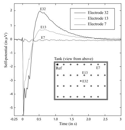
**Figure 4.** Electrograms for some selected electrodes (electrodes E32, E13, and E7) during the injection experiment (Experiment #1). Electrode E32 is located just above the source while electrode E7 is the furthest. Note the change of polarity on the electrograms of electrodes E32 and E13 at time t = 0.35 s.
