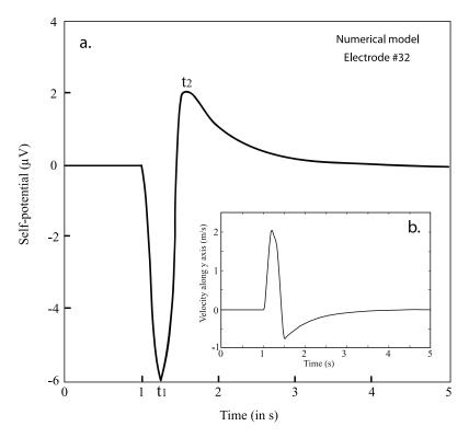
**Figure 14.** 2D numerical modeling of the self-potential response at electrode #32 (Experiment #1). (a) Note that the shape of the self-potential curve is similar to the measured self-potential signals (see Figure 4). (b) Computation of the fluid velocity at the end of the capillary. The reverse of the fluid velocity of the pore water is due to the fact that the fluid pressure is assigned equal to zero at t = 1.5 s.
