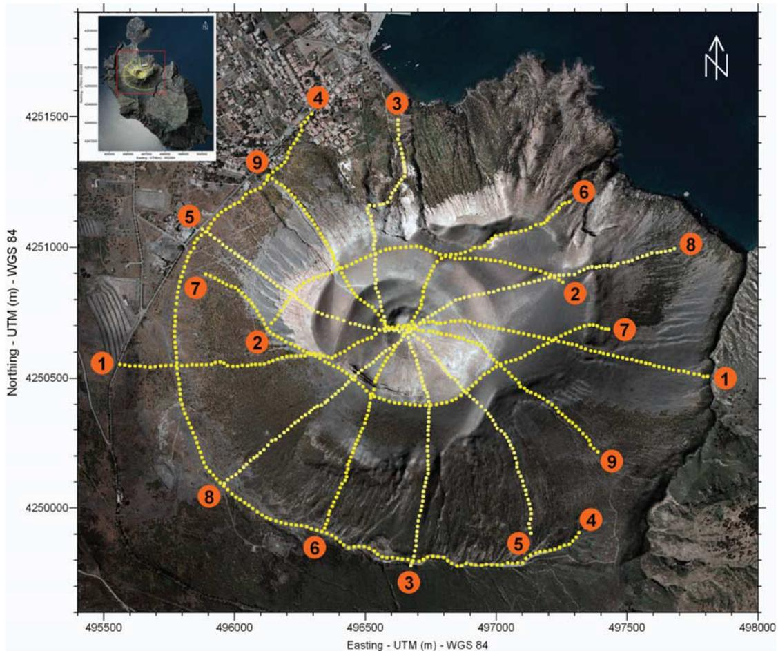
**Figure 2.** Position of the investigated area on the Fossa cone. Nine profiles (labeled from 1 to 9) have been performed crossing the Fossa edifice. The bright areas on the flanks of the volcano correspond to the hydromagmatic tuff discussed in the main text.
