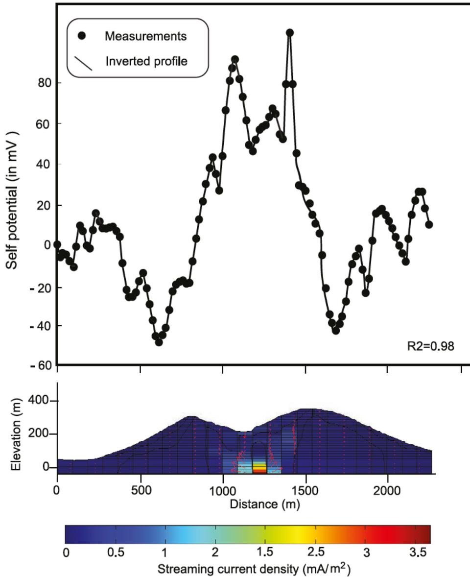
**Figure 16.** Inversion of the self-potential data in terms of the streaming current density. (a) Comparison between the measured self-potential data and the self-potential determined from the inverted model ( $R^2 = 0.98$ ). (b) Result of the inversion of the self-potential data with a depth weighting matrix and a derivative operator of order one. The arrows represent the direction of the current density vector.
