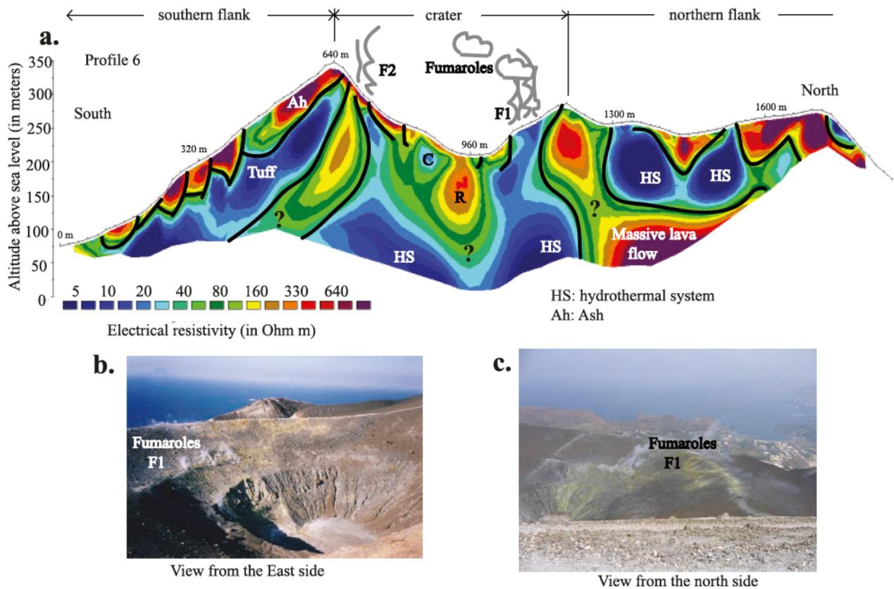
**Figure 12.** Architecture of the Fossa cone along the profile 6. The root of the area of fumarolic activity can be extended to a depth of 200 m below the ground surface. Abbreviations are as follows: F1 and F2, fumaroles; Ah, ash; HS, hydrothermal system. The internal part of the crater is characterized by a pocket of high conductivity (C) and a high resistivity structure (R).
