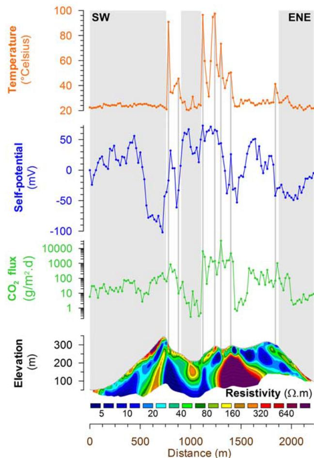
Figure 7. Temperature, self-potential, soil CO<sub>2</sub> flux, and electrical resistivity tomogram along profile 8.
