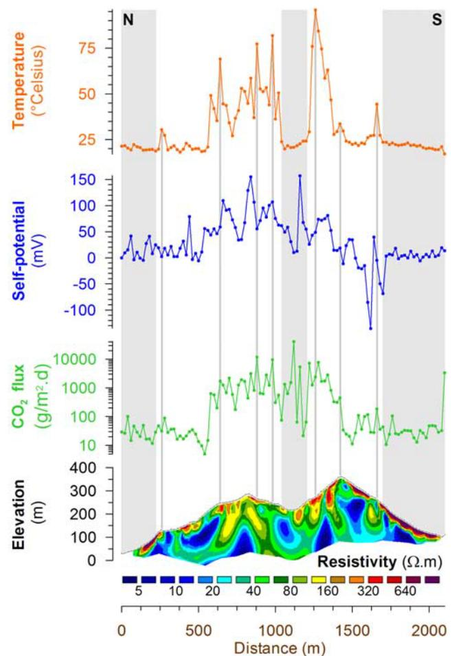
**Figure 5.** Temperature, self-potential, soil CO<sub>2</sub> flux, and electrical resistivity tomogram along profile 3. Note that the bottom part of the crater is cold. On the northern flank of the edifice (the left side of the figure), a conductive area is laterally limited by two thermal anomalies. These anomalies represent the boundary of the Forgia Vecchia crater which last eruption occurred in 1727.
