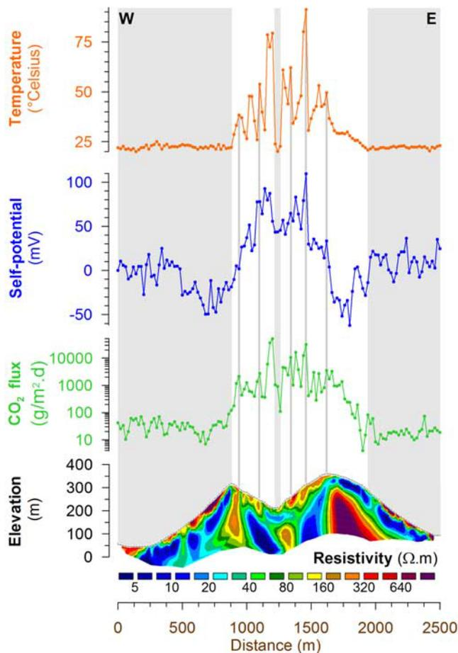
**Figure 4.** Temperature, self-potential, soil CO<sub>2</sub> flux, and electrical resistivity tomogram along profile 1. These data show that the main activity is constrained inside the crater, which is characterized by self-potential, CO<sub>2</sub>, and temperature anomalies. Note that the ground surface of the central part of the crater is cold.
