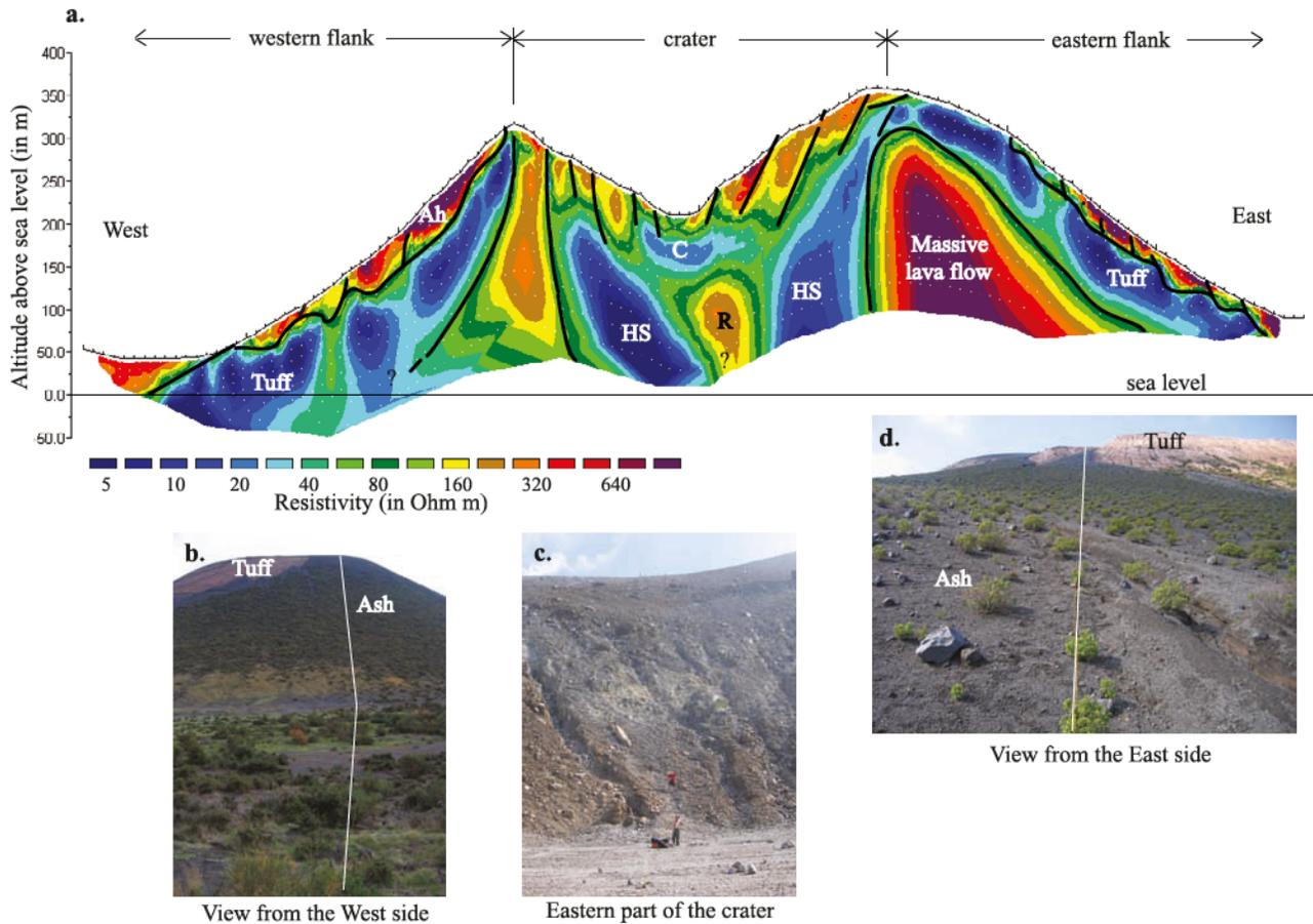
**Figure 11.** (a) Architecture of the Fossa cone along the profile 1 (resistivity tomogram). Abbreviations are as follows: Ah, ash; HS, hydrothermal system; C, conductive; and R, resistive. (b and d) Pictures of the Fossa cone from the west and east sides showing the position of the ashes relatively to the position of the hydromagmatic tuff (the line shows the position of the profile). (c) Picture taken inside the crater showing the pyroclastic deposits.
