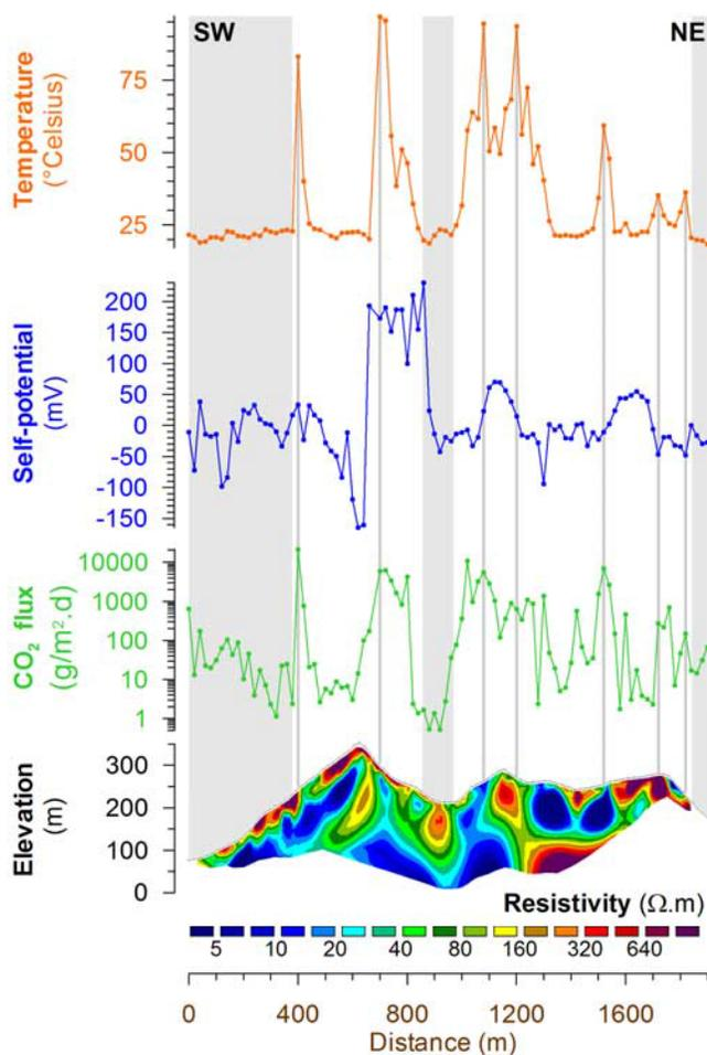
Figure 6. Temperature, self-potential, soil CO<sub>2</sub> flux, and electrical resistivity tomogram along profile 6. Note the M-shape of the temperature, self-potential, and CO<sub>2</sub> anomalies inside the crater.
