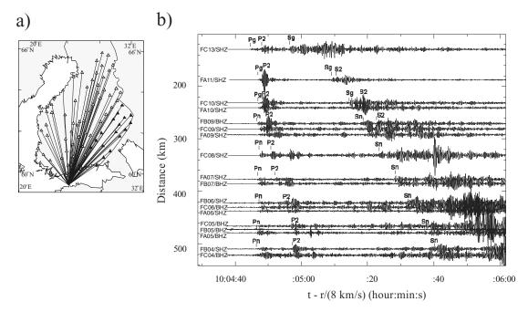
Figure 3. An example of a good quality event recorded by SVEKALAPKO array: (a) The  $M_L$  2.9 explosion offshore Estonia was recorded by 77 SVEKALAPKO stations on November 5th, 1998. Black triangles mark the stations from where the seismograms are shown. (b) The seismograms (3–6 Hz bandpass filtered) are presented in azimuth sector of 30°–60° from the epicentre. Crustal (Pg, Sg) and mantle (Pn, Sn)-wave arrivals and some distinct reflections (P2, S2) are marked above the recordings.
