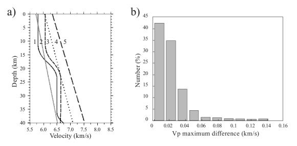
**Figure 4.** Testing *a priori* models. (a) Velocity-depth curves of five different *a priori* models: (1) IASPEI; (2) low velocity gradient; (3) model in Table 2; (4) model used in this study and (5) high velocity gradient. (b) Maximum differences (km s<sup>-1</sup>) in the velocity fields of the final inverted models are shown.
