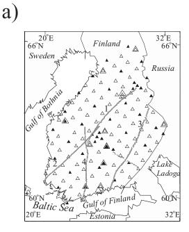
Seismic stations SVEKALAPKO sp △ bb▲ station Finnish permanent station △ DSS profile stations ✓ 1) SVEKA-81, 2) SVEKA-91, 3) BALTIC, 4) FENNIA b)
