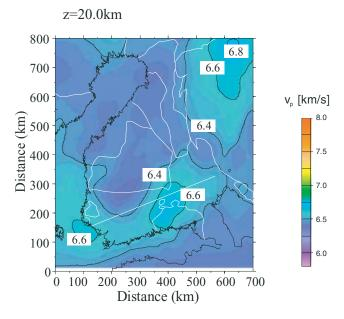
**Figure 9.** *P*-wave velocity model at depth of 20 km plotted from the velocity matrix of Sandoval *et al.* (2003) model (courtesy of Senen Sandoval). Corresponding depth slice of our model is shown in Fig. 6(a), z = 20 km.
