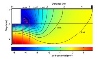
**Figure 5.** Simulated SP distribution and the Darcy velocity associated with the infiltration in the ditch of Roujan using all the hydraulic information available from in situ and petrophysical measurements [see *Bolève et al.*, 2007b].
