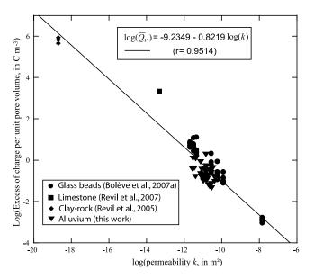
**Figure 1.** Dependence of the excess of charge per unit pore volume with the permeability at saturation of the porous materials. This data set includes various lithologies and salinities ( $6 \le pH \le 8.5$ ). The alluvium materials are from the Boise State University test site. They are composed of a mixture of sands and gravels.
