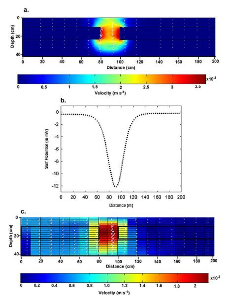
**Figure 3.** Synthetic case for a vertical 2D-infiltration problem. (a) True distribution of the Darcy velocity (in m s<sup>-1</sup>). (b) Distribution of the resulting self-potentials, which is sampled at the top surface of the system every meter. (c) Distribution of the reconstructed Darcy velocity ( $R^2 = 0.95$ ).
