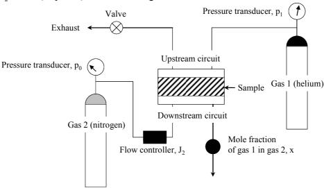
Figure 1: "Tracer" technique for the measurement of permeability.
