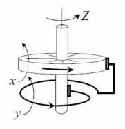
Figure 1: The homopolar (or Bullard) disk-dynamo.
