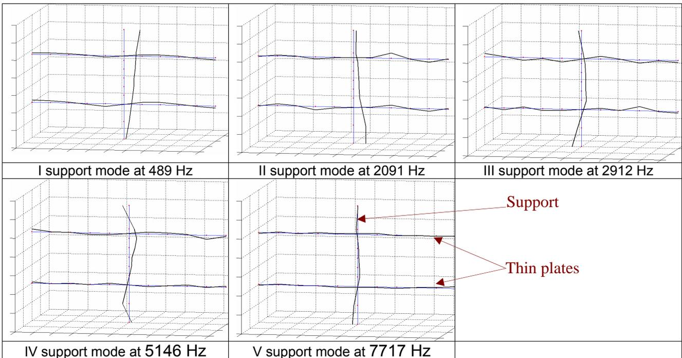
**Figure 3** – Deformed shapes of the support obtained experimentally.
