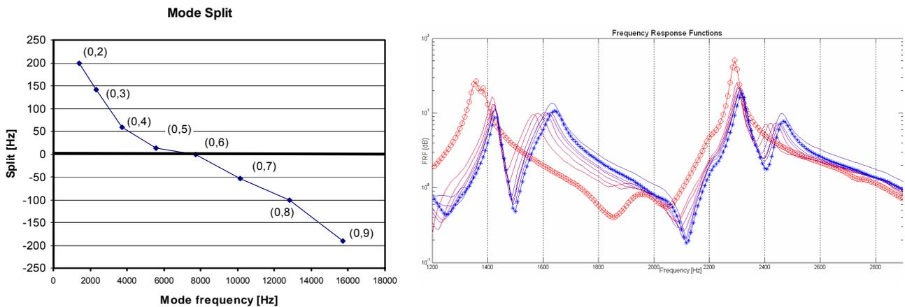
**Figure 5 - a)** Split of the disc modes with 225 N of normal load; **b)** Split of two and three nodal diameters modes in function of load: the red line (circles) is the FRF with no contact with the pad, the blue line (asterisks) is with maximum load.
