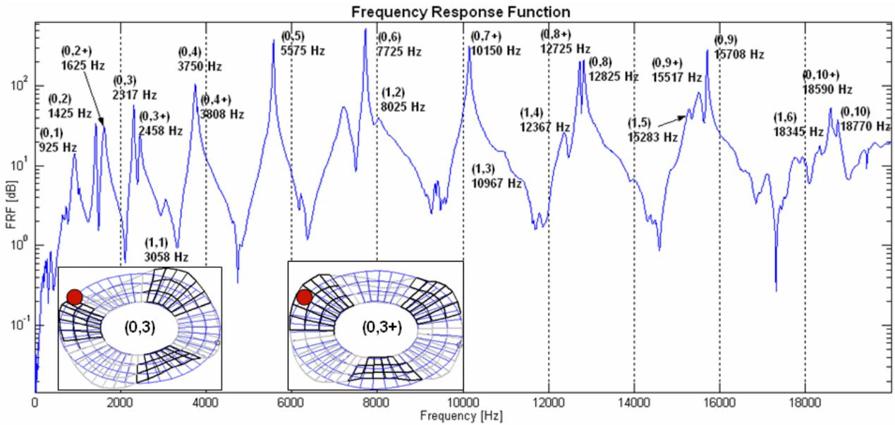
**Figure 2** - FRF of the set-up measured on the disc periphery, when a normal of 225 N is applied, and samples of the disc deformed shapes (0,3) and (0,3+). The big node is the contact surface with the pad.
