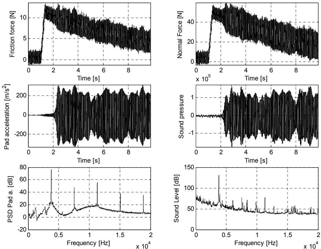
**Figure 6** – System vibration during squeal phenomenon at 3767 Hz.
