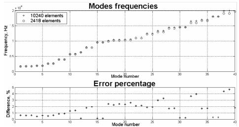
Figure 3: Error percentage between the eigenfrequencies obtained with the two meshes
