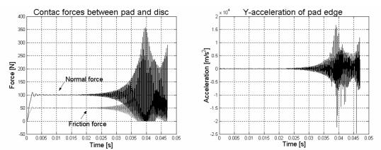
Figure 10:a) Sum of contact forces; b) Acceleration of pad edge in the friction direction for pad Young modulus equal to 39800 MPa – Plast3 simulation
