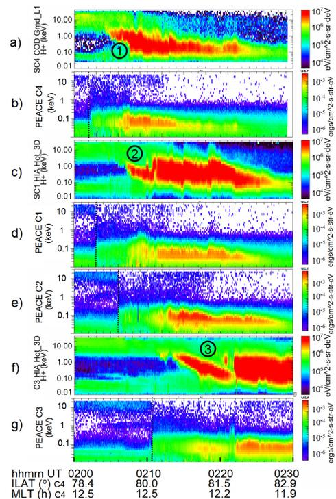
**Figure 2.** Omnidirectional ion and downgoing electron spectrograms on (a and b) C4, (c and d) C1, (e) C2, and (f and g) C3. Open-Closed Boundary is indicated by the dotted line on the electron spectrograms. The ion energy steps and dispersions are marked from 1 to 3.
