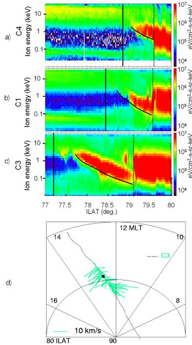
**Figure 3.** Omnidirectional ion spectrograms as a function of invariant latitude for (a) C4, (b) C1 and (c) C3. OCB is marked by a solid vertical line and the boundary between the energy steps/dispersion and the main cusp is marked by a dotted line. The solid lines mark the low-energy cut-off. (d) Flow speed from C3 in ILAT-MLT diagram. The star marks the boundary between the dispersion on the equatorward side of the cusp and the rest of the cusp poleward.
