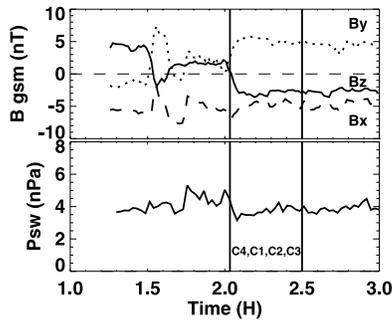
**Figure 1.** Solar wind conditions on 7 Aug. 2004 from the Wind spacecraft. A shift of 75 min was applied to the data to take into account the propagation from Wind position to the front of the magnetosphere. Bx is plotted with a dashed line, By a dotted line and Bz a solid line.
