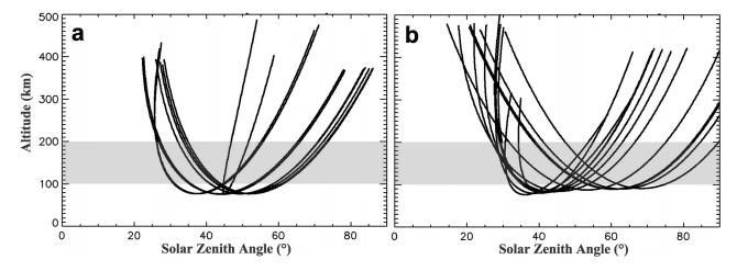
**Figure 2.** Traces of Mars Nearest Point of the FOV for the different period of observations selected from Table 2 plotted versus SZA and altitude. (a) Ten orbits during  $Ls = 100.95^{\circ} - 130.1^{\circ}$ . (b) Fourteen orbits during  $Ls = 138.56^{\circ} - 171.02^{\circ}$ .
