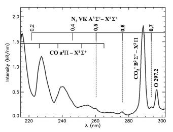
**Figure 13.** Spectrum of the Martian dayglow between 145 and 150 km in altitude, averaged from 2970 individual spectra measured by SPICAM (i.e., the whole set of observations described in this paper). The solar zenith angle range is between  $14^{\circ}$  and  $105^{\circ}$ , and the aerocentric longitude range is between  $100.95^{\circ}$  and  $171.2^{\circ}$ . Most of the plotted error bars are smaller than the thickness of the line.
