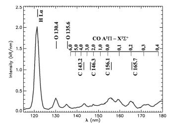
**Figure 5.** Spectrum obtained by SPICAM UV (the 100 - 180 nm spectral range) between SZA =  $14 - 37^{\circ}$  and Ls =  $135 - 171^{\circ}$  and between 140 - 150 km in altitude; 1224 individual spectra have been averaged. Most of the plotted error bars are smaller than the thickness of the line.
