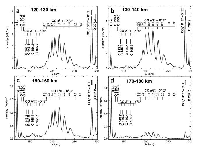
**Figure 6.** Spectra obtained by SPICAM UVS between SZA =  $14 - 37^{\circ}$  and Ls =  $135 - 171^{\circ}$ . (a) Average of 1102 individual spectra measured between 120 and 130 km. (b) Average of 1024 individual spectra obtained between 130 and 140 km. (c) Average of 1003 individual spectra obtained between 150 and 160 km. (d) Average of 1052 individual spectra obtained between 170 and 180 km. Most of the plotted error bars are smaller than the thickness of the line.
