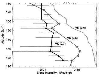
**Figure 14.** Variation of the intensity versus altitude (with 4-km altitude resolution) of the 260.4 nm emission feature, the (0,5) Vegard-Kaplan band (solid gray line with star), the 276 nm emission feature, the (0,6) Vegard-Kaplan band (solid gray line), and the 293.6 nm emission feature, the (0,7) Vegard-Kaplan band (solid dark line with diamond) for the entire set of observations described in this paper.
