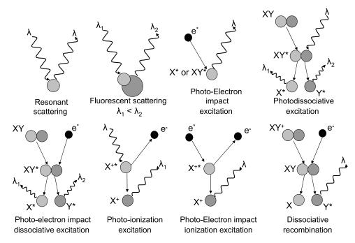
**Figure 1.** Scheme of the different mechanisms leading to the dayglow.  $\lambda$ ,  $\lambda_1$ , and  $\lambda_2$  are the wavelength of the incident or emitted photons. X and Y are atoms, and  $e^-$  is an electron;  $X^+$  or  $Y^+$  is for a positive ion, and X\*, Y\*, XY\*, or X<sup>+\*</sup> is an atom/molecule/ion in an excited state (adapted from *Paxton and Anderson* [1992]).
