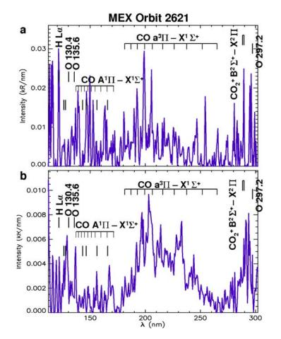
**Figure 1.** SPICAM ultraviolet spectrograph (UVS) spectra of the aurora event during orbit 2621. (a) As measured with the spatial bins facing the narrow part of the slit (best spectral resolution) during 14 s. (b) As measured with the spatial bins facing the large part of the slit (lowest spectral resolution). Each spectrum is the average of the 28 individual spectra measured during this event on the two spatial bins (14 each) either with the worst spectral resolution or the best one.
