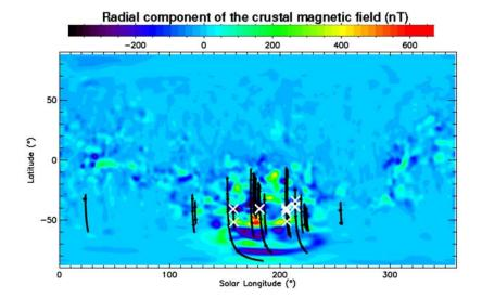
**Figure 3.** Trajectories of Mars Express during nadir viewing observations by SPICAM UVS. Only the part of each orbit with the spacecraft below 1000 km in altitude has been plotted. These trajectories are plotted on a 2-D map of the radial component of the Martian magnetic crustal field as calculated at 200 km in altitude [*Purucker et al.*, 2000]. The positions of the identified aurora during these nadir viewing orbits are also plotted with white crosses.
