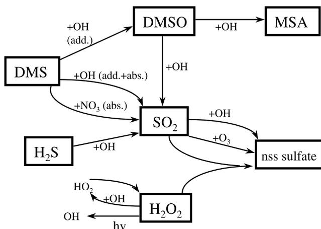
**Figure 2.** Chemistry scheme used in LMD-ZT. Details of the kinetics are presented by *Cosme et al.* [2002]. Here, “add.” and “abs.” refer to the addition and abstraction channels of DMS oxidation, respectively.  $\text{SO}_2$  oxidation by  $\text{O}_3$  and  $\text{H}_2\text{O}_2$  occurs in the aqueous phase.
