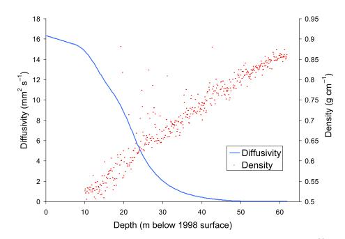
**Figure 9.** Diffusivity profile for Devon Ice Cap firn, produced by inverse modeling with <sup>14</sup>CO<sub>2</sub>, shown with density data measured on the Devon 98-1 core.
