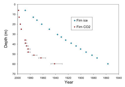
**Figure 7.** Reconstructions of the age structure of firm ice based on the rate of burial of the 1963 atmospheric tritium peak, and mean age of firm air based on <sup>18</sup>O exchange between  $CO_2$  and firm ice in the Devon 98-1 drill hole. Error based on the range in  $T^{1/2}$  from uncertainties in the depth of the 1963 peak (±1.5 m).
