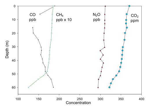
**Figure 3.** Trace gas concentrations in firm air sampled in the Devon 98-1 drill hole on the Devon Island Ice Cap.
