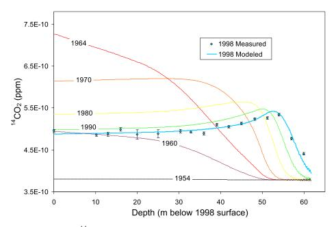
**Figure 10.** Modeled 1998 <sup>14</sup>CO<sub>2</sub> profile compared with measured values from firn air in the Devon 98-1 core hole, together with modeled profiles for earlier decades showing the evolution of the <sup>14</sup>CO<sub>2</sub> profile since the period of atmospheric tests.
