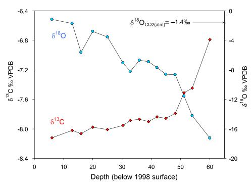
**Figure 5.** Depth profiles for the stable isotopic content of CO<sub>2</sub> (uncorrected for gravitational settling and diffusion) in Devon 98-1 firn air. Anomalous values for  $\delta^{18}$ O at 15.95, 30.33, and 32.85 m are due to ethanol contamination during analysis.
