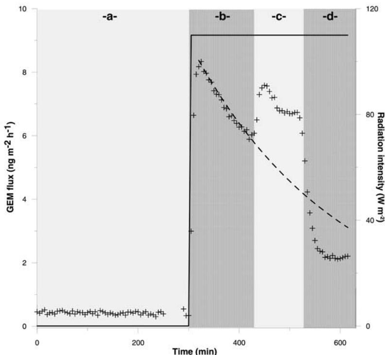
**Figure 6.** Variation of GEM flux ( $\text{ng m}^{-2} \text{h}^{-1}$ ) with time measured in the laboratory flux chamber. Phase a reports dark flux at  $-4^{\circ}\text{C}$ . During phase b, c and d, total irradiation was  $120 \text{ W m}^{-2}$  with wavelengths above  $295 \text{ nm}$ . Temperature in the chamber was kept at  $-4^{\circ}\text{C}$  during phase b, and then increased to  $+1.5^{\circ}\text{C}$  during phase c and d.
