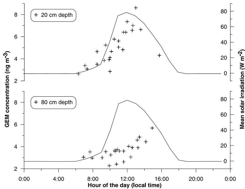
**Figure 2.** Variation of GEM concentrations in the snowpack ( $\text{ng m}^{-3}$ ) at 20 and 80 cm depth with time. All data obtained during the field campaign are reported. Solar radiation is the mean calculated for the entire measurement period.
