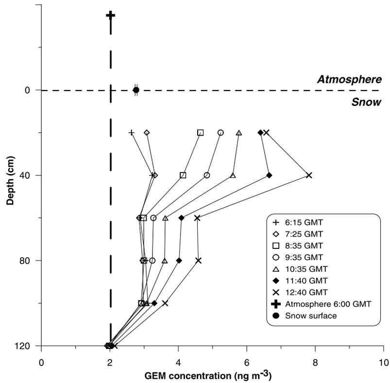
**Figure 1.** GEM profiles in interstitial snow air from the surface to 120 cm depth on March 15. Surface concentration reported here is an average of 20 measurements obtained the same day between 1:00 and 3:00 pm. The atmospheric level is the concentration determined at 6:00 am before sunrise. The error bar reported at the surface is one standard deviation of the mean values.
