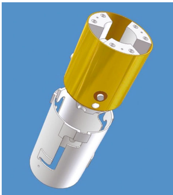
Fig. 10. Bayonet coupling or the super banger. The upper block is attached to the lower end of the hollow shaft, and the sleeve is welded to the top of the core barrel. The three rollers on the block can be latched on, inside the grooves of the sleeve. This way the core barrel can be mounted on or released from the drill at the bottom of the hole or at surface. Another feature can provide heavy impact on the core barrel by pulling hard on the drill with the rollers in the lower left (normal) position and then rotating the drill backwards. This feature still needs to be properly tested but could help to release stuck drills as the main mass of the drill is acting as a hammer.
