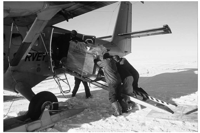
Fig. 6. Unloading the winch frame from the Twin Otter using H-section ramps.
