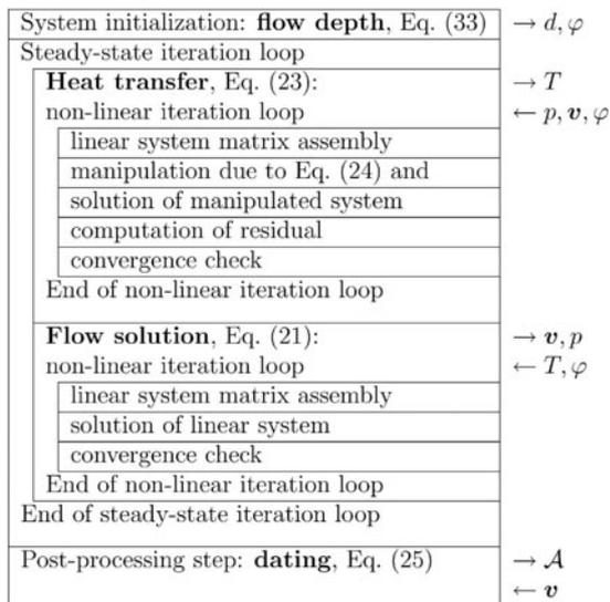
**Fig. 4.** Flowchart of the numerical simulations. Symbols behind leftwards pointing arrows indicate the needed input variables, whereas rightwards pointing arrows depict solution variables for the different modules.
