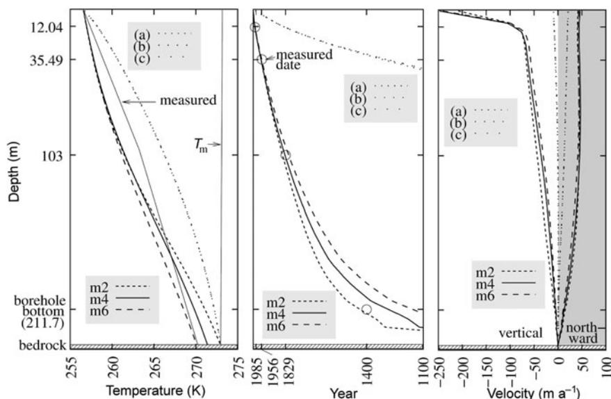
**Fig. 8.** Profiles of simulation results at the K2 drill-site: (a) temperature; (b) age profile and (c) vertical and northward velocity. Measured temperature profile and age points by Shiraiwa and others (2001).
