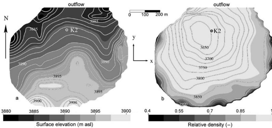
**Fig. 1.** (a) Surface topography of the Gorshkov crater glacier (greyscale texture and contours, contour spacing 1 m); (b) Bedrock topography (contour, spacing 25 m) and basal relative density (greyscale texture).
