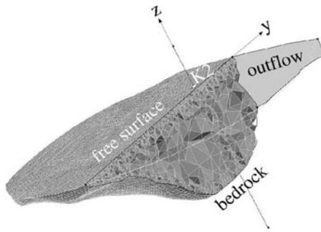
**Fig. 2.** Cut through the computational mesh of the Gorshkov crater. The black vertical line indicates the position of the borehole K2. The three boundary areas, namely the free surface, bedrock and outflow, are indicated.
