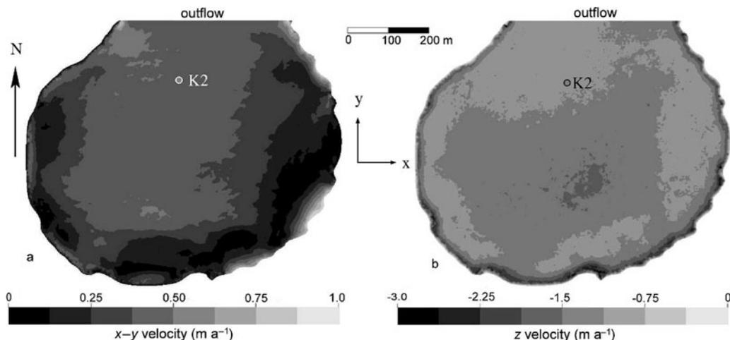
**Fig. 5.** Near-surface velocity (at 10 m depth) for the reference run ( $m4$ ) (a) absolute value of the horizontal ( $x$ - $y$  plane) velocity; (b) absolute value of the vertical velocity ( $z$ -direction).
