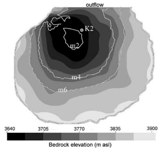
**Fig. 7.** Regions of cold and temperate basal ice (inside and outside of the white contour lines, respectively) for the reference run (*m4*), the run (*m2*) and the run (*m6*). The bedrock elevation is underlaid as greyscale texture.
