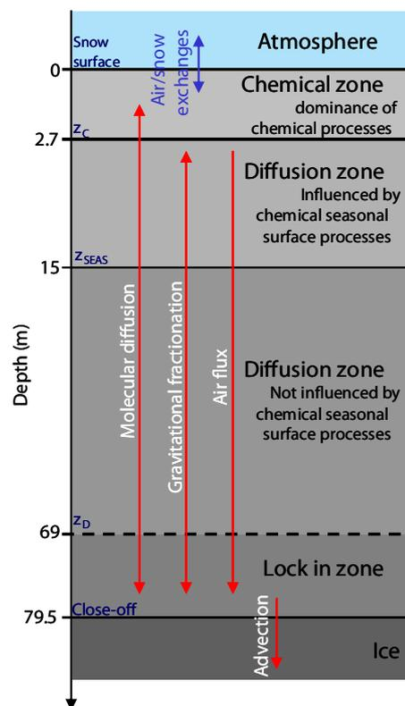
**Fig. 8.** Schematic view of the firn at Summit Station. Chemical processes involving GEM were observed in the Chemical Zone close to the surface. Below, the Diffusion Zone is characterized by physical transport mechanisms of GEM.
