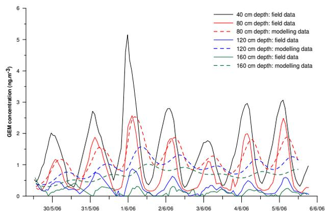
**Fig. 6.** Modeling of diffusion with depth of GEM variations observed at a depth of 40 cm in June 2006. The dashed lines represent the field observations, while the full lines represent the expected variations if only diffusion was happening in the SIA.
