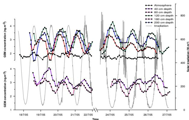
**Fig. 4.** GEM concentrations 1.5 m above the snow surface and at 40, 80, 120, 160 and 200 cm depths in the SIA, from 18 to 27 July 2005, at Summit Station. The grey line reports the global irradiation ( $\text{W m}^{-2}$ ).
