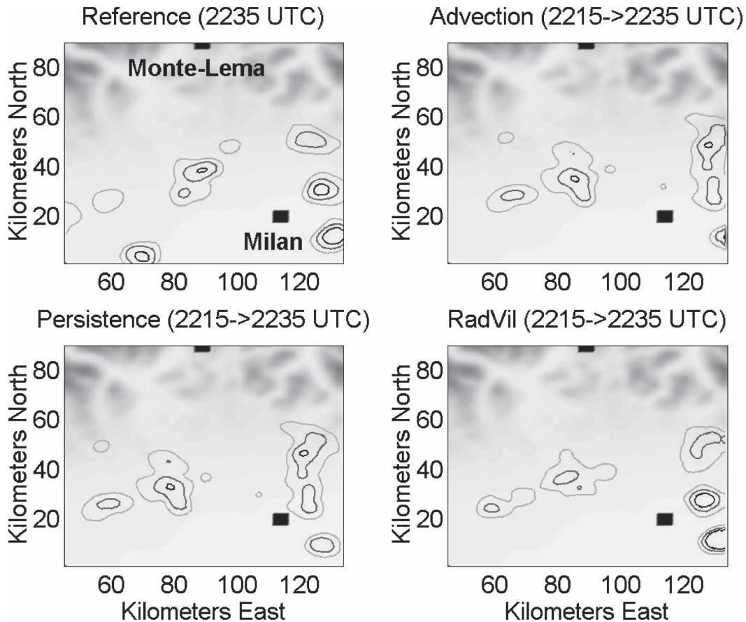
FIG. 3. Qualitative evaluation of RadVil on the first case study (17 Sep 1999):  $x$ - $y$  plot of the (top left) reference rainfall at 2235 UTC, and (bottom left) the forecast of the persistence model (equal to the reference field at 2215 UTC), (top right) the advection model, and (bottom right) RadVil for 2215 UTC + 20 min. The  $x$  and  $y$  axes are given in km. The rainfall isohyets are contoured with spacings of 10, 20, 30, and 40  $\text{mm h}^{-1}$ .
