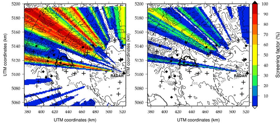
**Fig. 4.** Screening factors expressed in percent of the transmitted power for the lowest elevation angles ( $0.5^\circ$  left;  $1^\circ$  right). Note that the watershed of interest is severely masked in its southern part.
