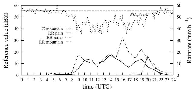
**Fig. 2.** Time series of the mountain reference target value (dashed line on top), the average rainrate along the path (bottom part of the graph, continuous line), the rainrate in the vicinity of the mountain (dash-dotted line) and the rainrate close to the radar site (dotted line).
