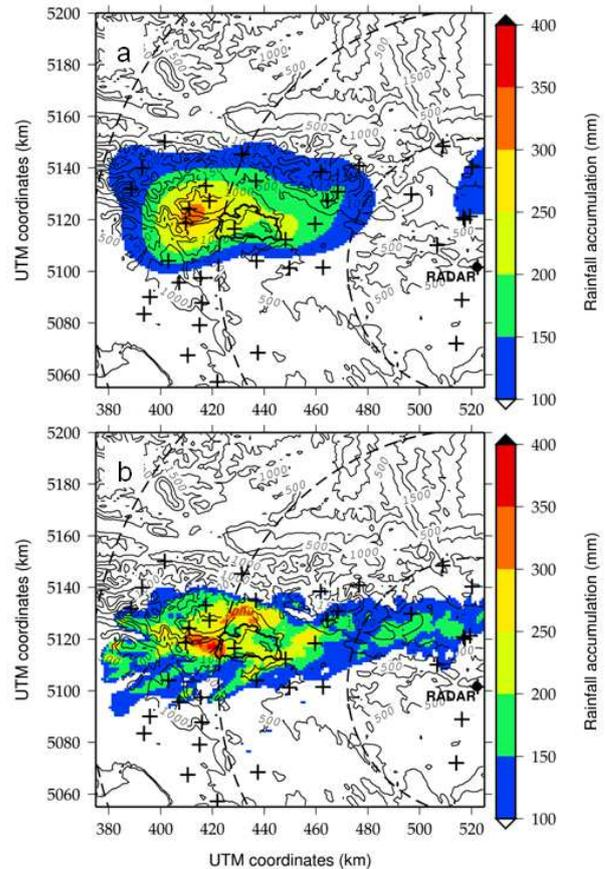
**Fig. 7.** Raingauge (a) and radar (b) rainfall fields at the event time scale for rainfall values greater than 100 mm. The radar estimates are obtained with the MRT technique by considering the Cévennes DSD parameterization and a PIA threshold of 10 dB.
