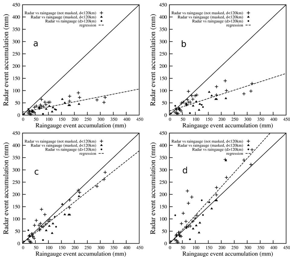
**Fig. 6.** Scatterplots of radar estimates versus raingauge measurements at the event time scale with the following radar data processing: **(a)** screening and VPR correction of the raw reflectivity; **(b)** in addition, the  $\delta_C$  correction is performed; **(c)** in addition, the attenuation correction is performed with a maximum corrected PIA of 10 dB; **(d)** same as (c) with a maximum corrected PIA of 20 dB. The Cévennes  $(Z, k, R)$  relationships are used.
