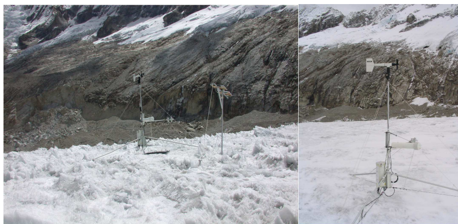
Fig. 2. The automatic weather station (SEBS) on the tongue of Glaciar Artesonraju in August 2005 when this study was made (left, photo: M. Winkler), and in July 2004 (right, photo: P. Wagnon). The difference in surface roughness is evident. In August 2005 a rough, undulated surface with many penitentes and cryoconite holes was dominant, in July 2004 the surface was much smoother.
