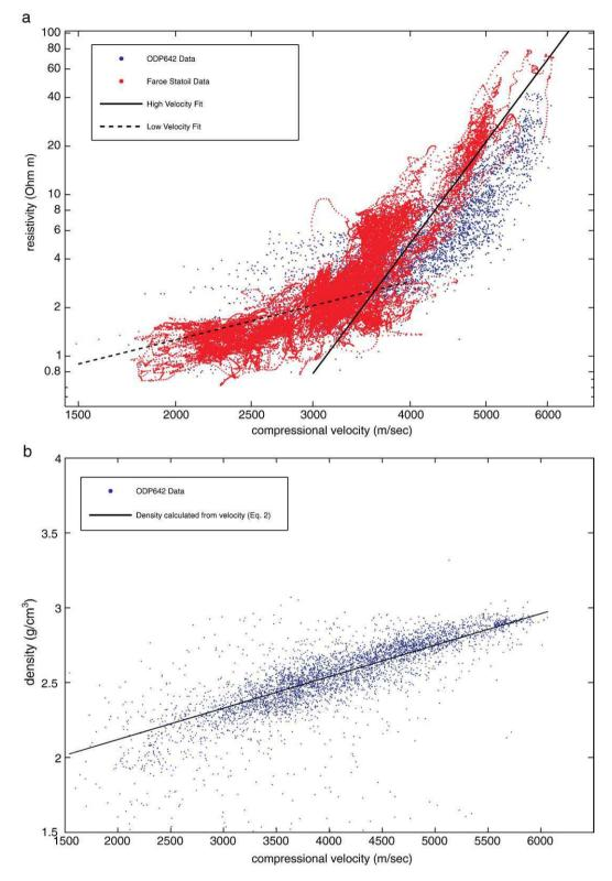
Fig. 1. a) Compressional velocity versus electrical resistivity for ODP642 borehole in the Voring basin and a Statoil borehole off the Faroe shelf. Solid and dotted lines denote relationship between velocity and electrical resistivity derived from linear fits of borehole data for low and high velocities. b) Compressional velocity versus density for ODP642 borehole in the Voring basin. Solid line denotes relationship between velocity and density derived from linear fit.
