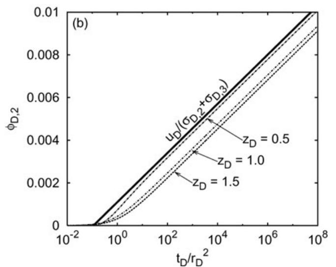
**Figure 3.** (a) Log-log and (b) semi-log plot of the dimensionless streaming potential response of the upper confining unit,  $\phi_{D,2}$ , against  $t_D/r_D^2$  for different values of  $z_D$  with  $\sigma_{D,2} = \sigma_{D,3} = 10^3$ .
