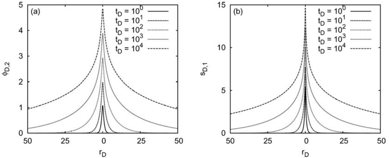
**Figure 4.** Plot of (a) the dimensionless streaming potential response of the upper confining unit,  $\phi_{D,2}$ , and (b) the dimensionless drawdown in the aquifer,  $s_{D,1}$ , against dimensionless radial distance,  $r_D$ , at different values of dimensionless time,  $t_D$ .
