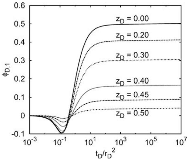
**Figure 2.** Semi-log plot of the dimensionless streaming potential response of the aquifer,  $\phi_{D,1}$ , against  $t_D/r_D^2$  for different values of  $z_D$  with  $\sigma_{D,2} = \sigma_{D,3} = 10^3$ .
