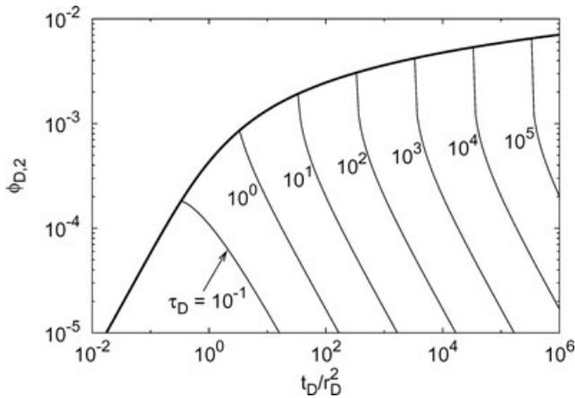
**Figure 5.** Log–log plot of the dimensionless streaming potential response of the upper confining unit,  $\phi_{D,2}$ , against  $t_D/r_D^2$  for different values of  $\tau_D$  with  $\sigma_{D,2} = \sigma_{D,3} = 10^3$ .
