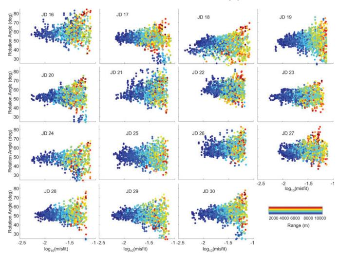
Figure 5. Day-by-day representation of the optimal azimuthal rotation angle  $\psi$ m versus the optimal rotation misfit for each station pair. Misfit values were calculated as the total energy on components ZT, TZ, RT and TR of the optimal noise-correlation tensor  $[\tilde{C}_{AmBm}(t)]_{ij}$  normalized according to the total energy of all of the components. The colour scale corresponds to the range between station pairs.
