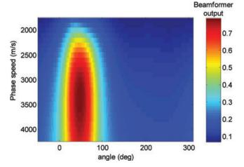
**Figure 2.** Angular-speed distribution of pre-processed incoming noise on the Parkfield network averaged over 1 d. Plane-wave beam-forming is summed incoherently over 100 frequencies from 0.1 to 0.2 Hz. The *x*-axis corresponds to noise directivity  $\theta_0$  (North is  $0^{\circ}$ , positive rotation is clockwise), the *y*-axis to speed *c*. Units are arbitrary.
