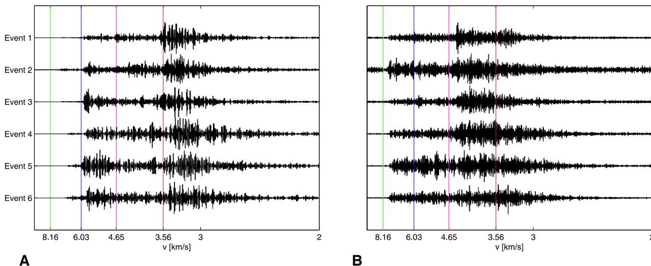
**Figure 7.** Seismograms of six earthquakes recorded within (a) the zone that blocks Lg waves and (b) recorded after the waves passed through this zone. A map showing the locations of the events and the stations is shown in Figure 8.
