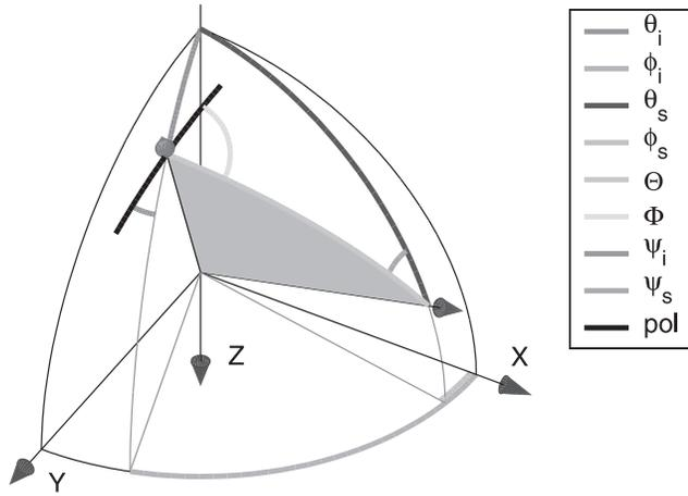
**Figure D1.** Illustration of the scattering and the polarization angle and their relation to the global polar coordinate system. Red and blue arrows indicates the directions of the incoming and scattered particle, respectively. The polarization direction of the incoming S particle is indicated by the bold black line.
