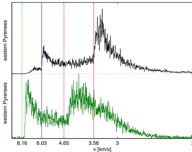
**Figure 9.** Reference traces from the eastern and western Pyrenees. Vertical lines indicate arrival times of seismic phases. The upper black trace represents undisturbed propagation through the eastern Pyrenees. It shows clear arrivals of crustal phases. The bottom trace represents wave paths through the western Pyrenees. Here the crustal phases are attenuated and only the mantle phases show clear arrivals.
