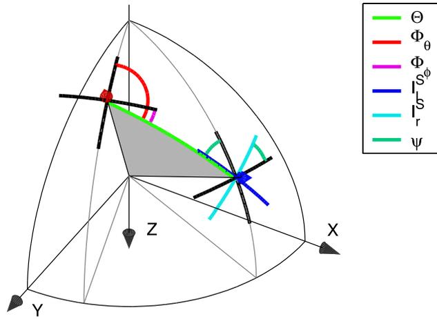
**Figure 3.** Illustration of the S polarization directions in the radiative transfer equations. Angles are identified by color of the arcs. The red and blue arrows indicate directions  $n'$  and  $n$ , respectively. The blue lines labeled  $I_l^S$  and  $I_r^S$  indicate the directions of polarization of the parallel and perpendicular intensity components, respectively.
