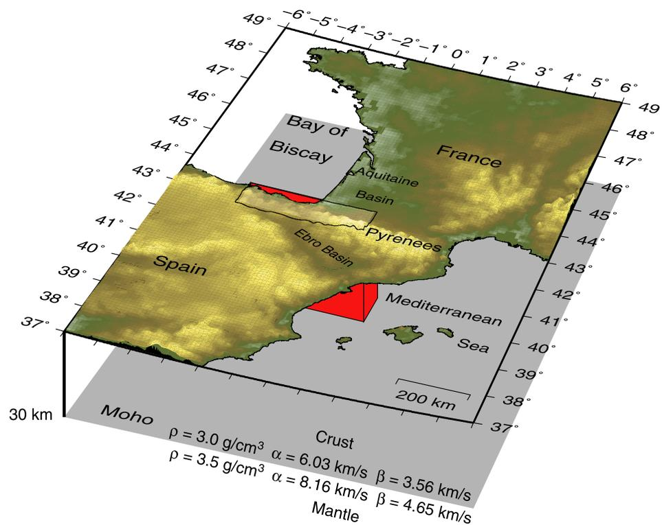
**Figure 4.** Map of the study area and illustration of the model that is used to explain the Lg blockage in the western Pyrenees. The gray plane and the red box depict the Moho and the region of increased heterogeneity, respectively. The parameters of the model are indicated. In the mantle the P wave velocity increases with depth by  $d\alpha/dz = 300 \text{ s}^{-1}$ .
