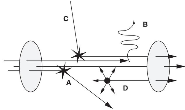
**Figure 1.** Illustration of the energy conservation in the energy transfer equation. The flux in direction  $\mathbf{n}$  is diminished by scattering into other directions (A) and by dissipation (B). A gain of the flux results from scattering from other directions into direction  $\mathbf{n}$  (C) and from sources (D).
