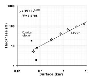
**Fig. 2.** Relationships between glacier surface area and mean thickness. Grey diamonds and equation indicate the relationship given by Marangunic (1979); black squares represent three glacierets and one glacier in the Huasco valley computed from GPR measurements made by Golder Associates as part of the glacier monitoring program of the future Pascua-Lama mining project (Barrick Gold Corporation).
